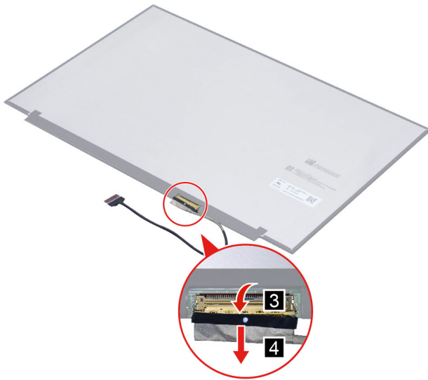
Figure 29. Remove the EDP cable
