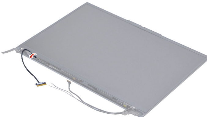
Figure 26. Release the EDP cable
