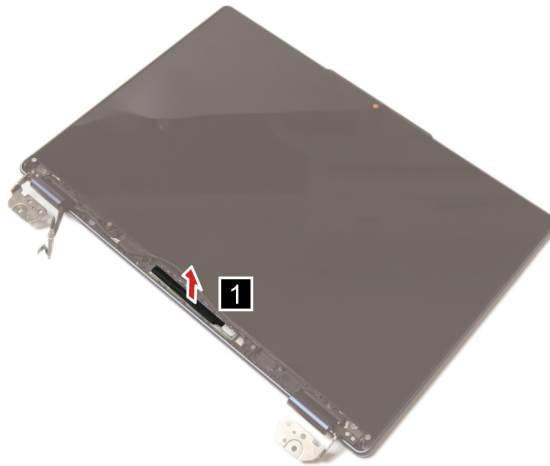
Figure 27. Remove the acetate tape
