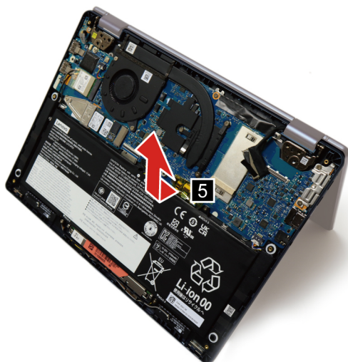
Figure 25. Remove the upper case (with keyboard)
