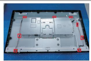
Unplug OSD key cable and tear off the tape for releasing the cable
