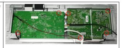
Remove the pins and boards
