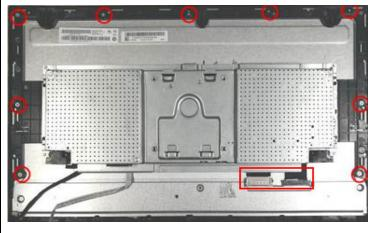
Separated the panel and the middle frame. The panel The middle frame Take off the taype and the mylar. Remove the screw\*6pcs to remove the Main board and the power board.
