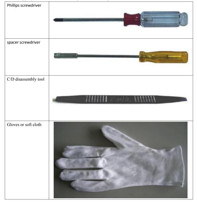
Select the Appropriate tools for disassembly and re-assembly.
