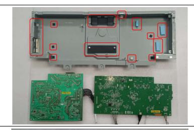
Remove screws\*10pcs to take out the Front bezel.
