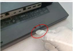
Remove the chassis screws (red);
