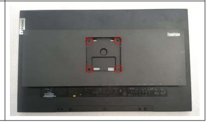
Use the C/D disassembly tool to release Rear cover hook from disassemble hole on bottom.
