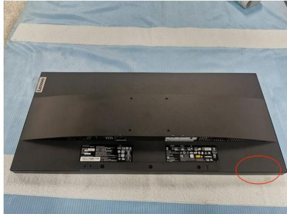
Disassemble the back cover, take out the speaker cable at the side of the isolation cover, and take down the back cover
