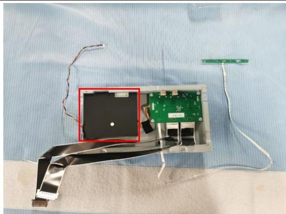
Remove the main board and power board screws
