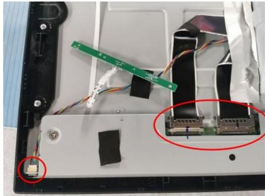
Remove the black Mylar from the power board
