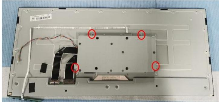
Remove the lamp wire and FFC wire
