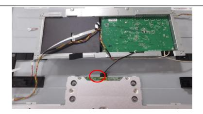
Remove the mylar sheet on the power board
