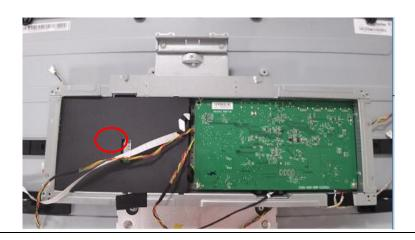
Unscrew the 6\*screws on the boards
