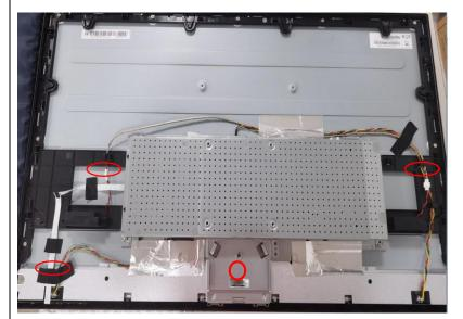
Turn over the mainframe and disconnect the connectors as the picture
