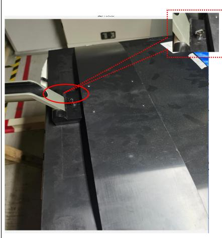
Use the C/D disassembly tool to release Rear cover hook from the bottom site
