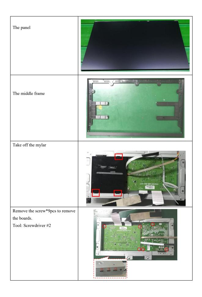
Remove the pins and boards
