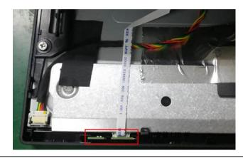
Remove the screw\*9pcs to separate the panel and the middle frame.
