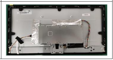
Remove All screw. Tool: Screwdriver #2 Release the middle frame from the Panel Release the keypad pcb from the the middle frame Unplug light bar line and LVDS line Remove the acetate tape Take out the mylar sheet from Main chassis
