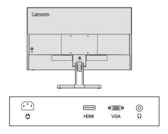
3. Connect one end of the VGA cable to the VGA connector on the back of the computer, and the other end to the VGA connector on the monitor.
