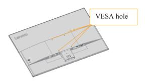
Step 5: Attach the LCD display to the wall, and follow the instructions in the wall-mounting kit. For use only with UL Listed Wall Mount Bracket with minimum weight/load: 8kg
