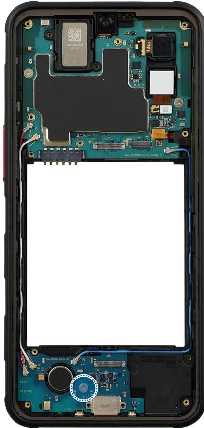
4 Place the upper part of bracket on the device frame and push down all edges of the bracket using your fingers softly and evenly so that the bracket can be assembled perfectly.
