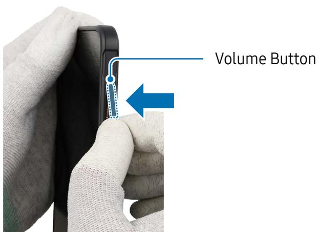
2 Press down the Volume button softly and evenly so that the button can be completely assembled. Press the Volume button to make sure it clicks. It should have the same sound and feel as before disassembly.
