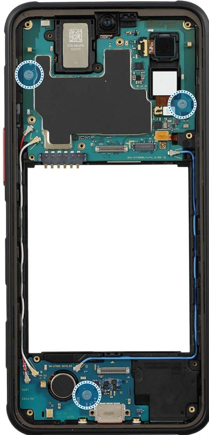
3 Separate 2 connectors of the coaxial cable (White) with the tweezers and remove the cable (White) from the device frame.
