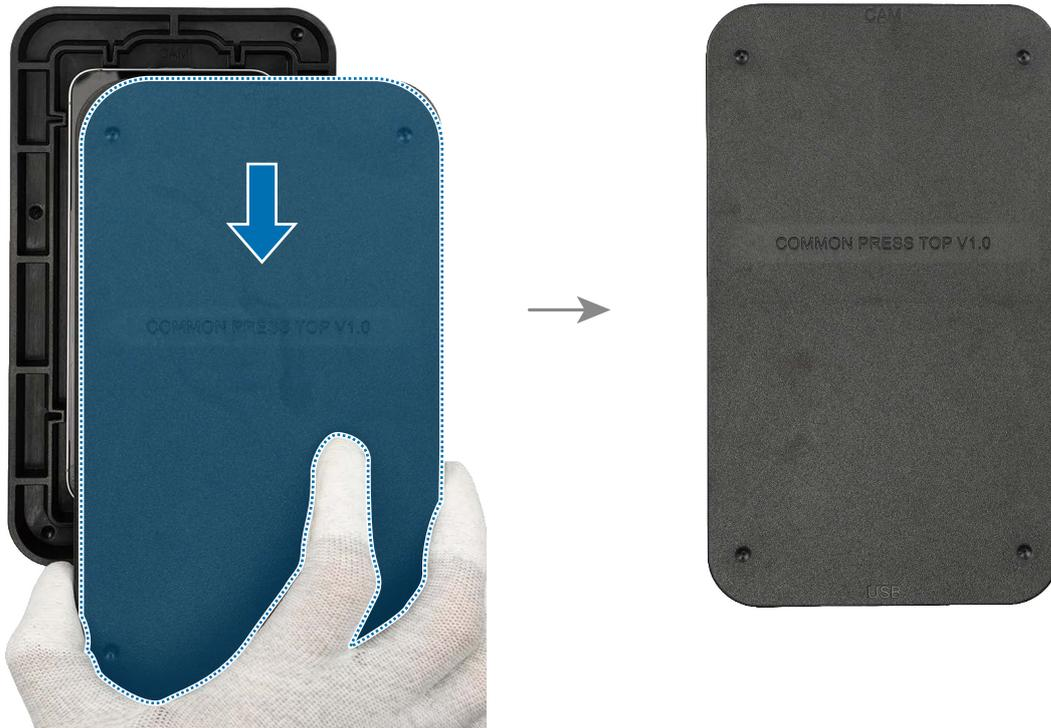
14 Position the top 2/3 of the screen press tray with the device lengthwise in the centre of the press fixture.
