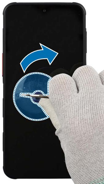
3 While pulling up the suction cup with strong, steady force to create the gap between the screen and the frame, place the opening pick in the gap and slide the opening pick back and forth along the edge to slice through the adhesive. Repeat this on the all sides of the screen and slice through the adhesive. Lift up from the top of the screen slowly and remove the screen gently from the device.
