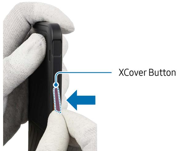
4 Press down the XCover button softly and evenly so that the button can be completely assembled. Press the XCover button to make sure it clicks. It should have the same sound and feel as before disassembly.
