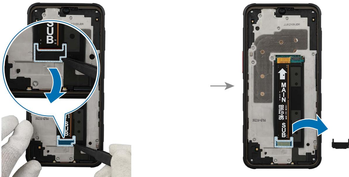
2 Using the tweezers, disconnect the 2 flex cable connectors and remove the flex cable completely.
