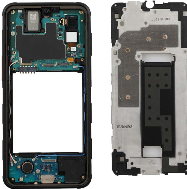
2 Check the 2 screws on the main board and remove them using a cross-head screwdriver.
