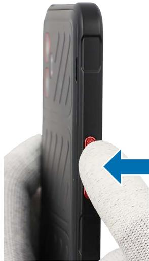
5 Remove the release film of the new Emergency button. Use your fingers to grab the Emergency button and insert the button on the slot carefully.
