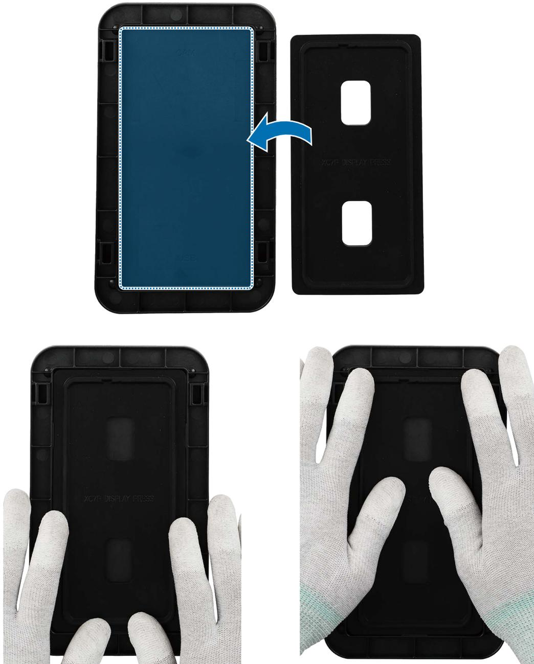
13 Carefully place the top press tray over the bottom press tray.
