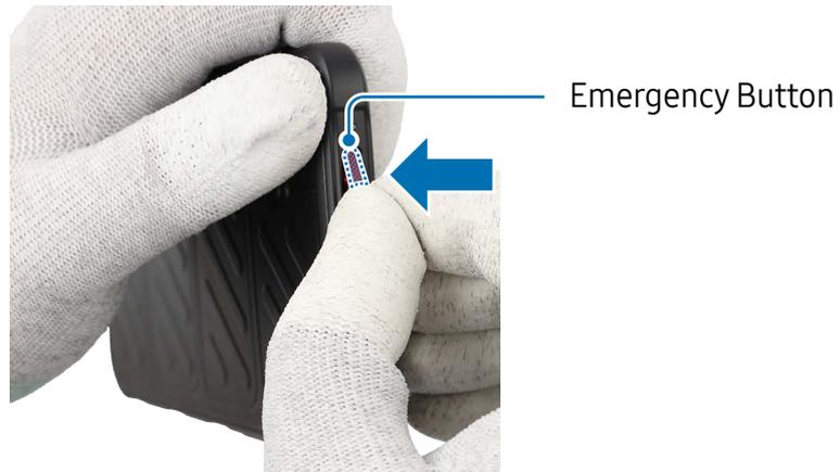
6 Press down the Emergency button softly and evenly so that the button can be completely assembled. Press the Emergency button to make sure it clicks. It should have the same sound and feel as before disassembly.
