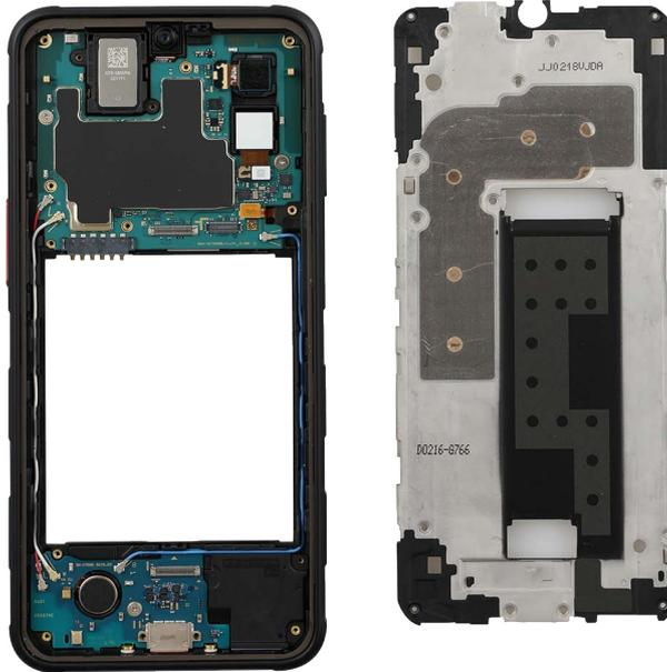
2 Disconnect the rear camera connector from the main board using the tweezers, and remove the rear camera carefully from the main board. Leave the camera lens facing up.
