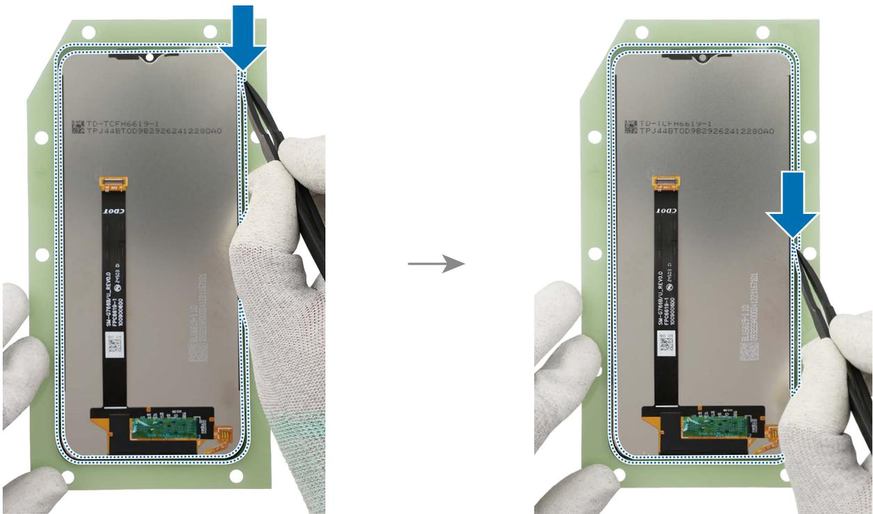
4 Using the tweezers, remove all release films from attached tape.
