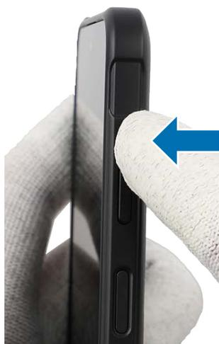
3 Remove the release film of the new XCover button. Use your fingers to grab the XCover button and insert the button on the slot carefully.
