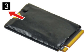
Figure 10. Remove the SSD foil from the SSD
