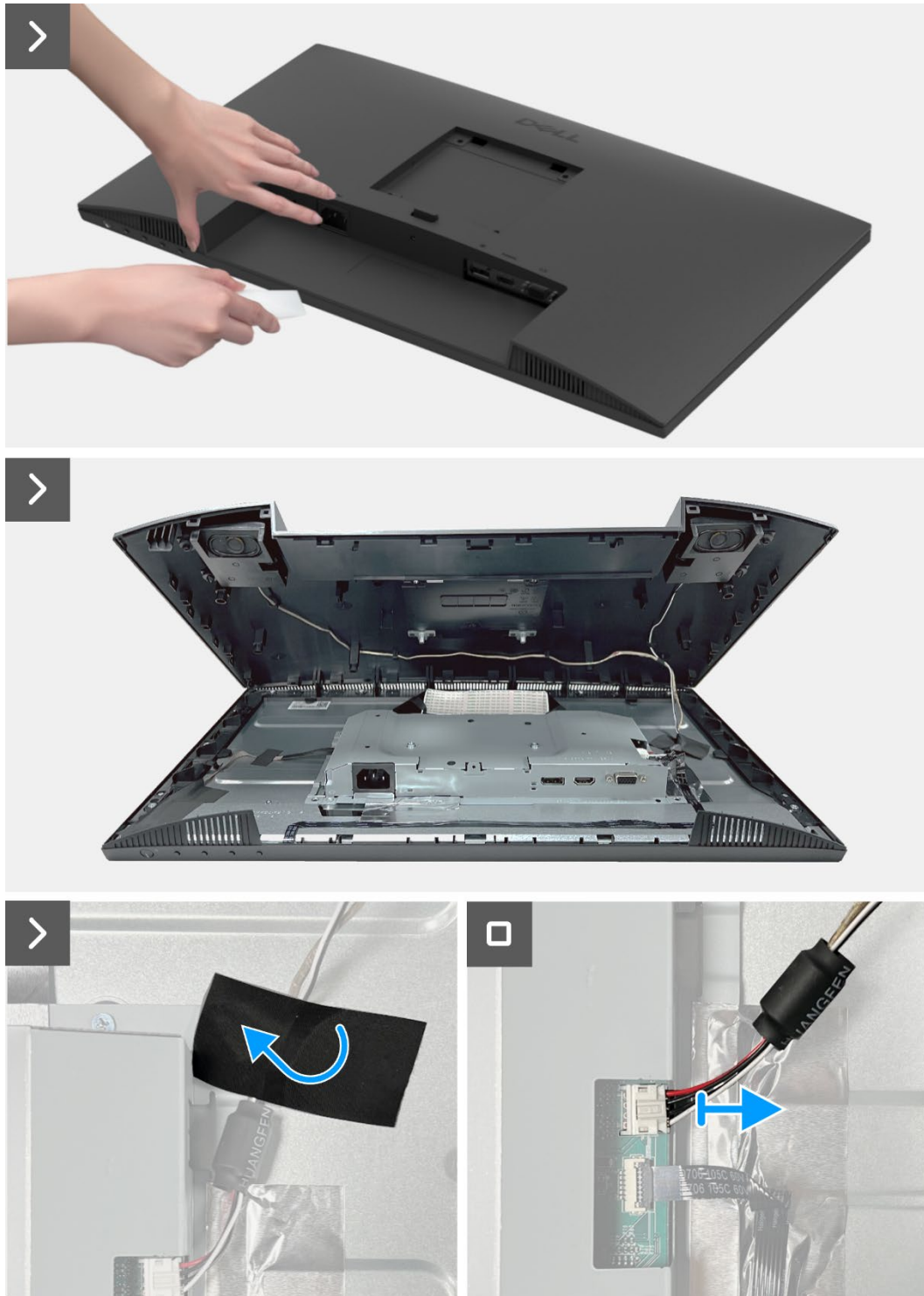
Figure 35. Removing the back cover
