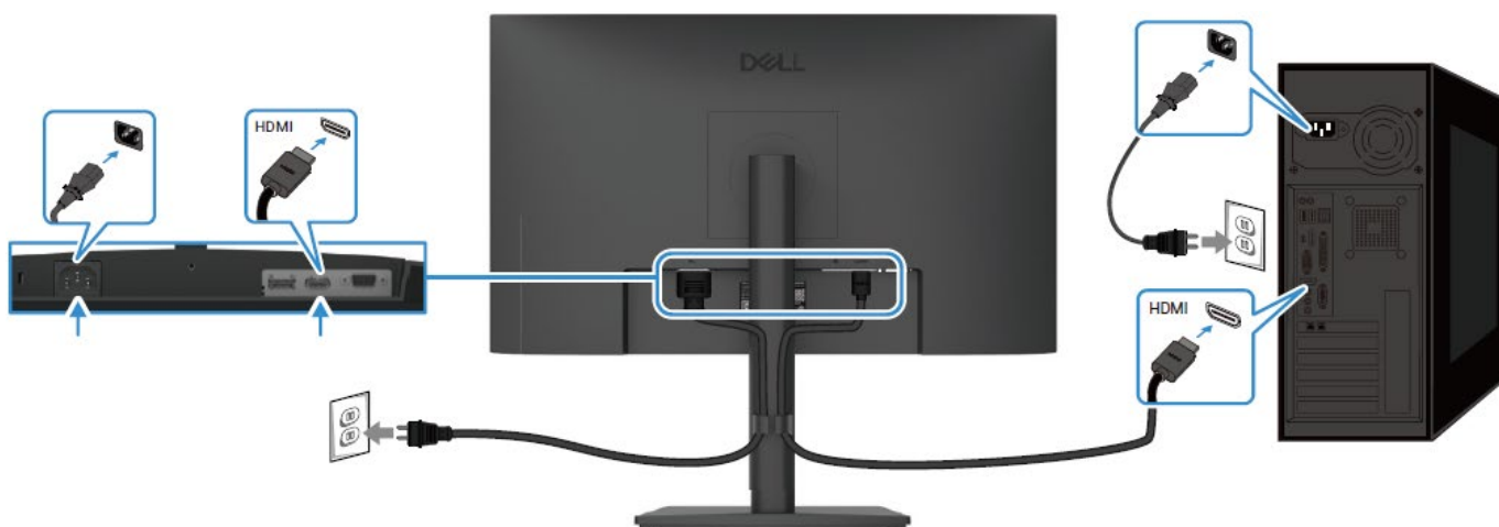
Figure 9. Connecting HDMI cable
