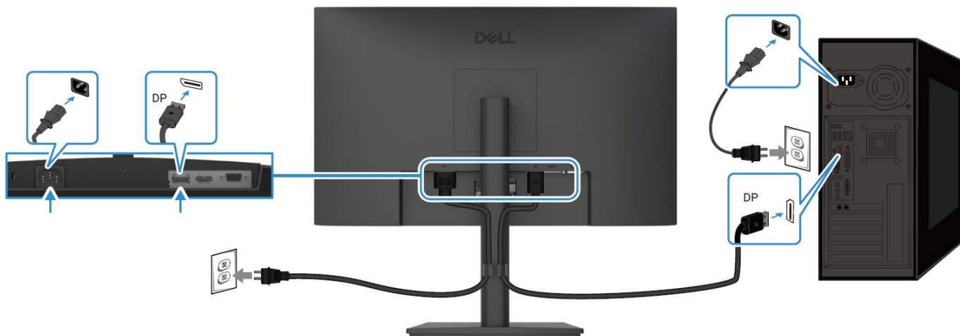
Figure 8. Connecting DP cable
