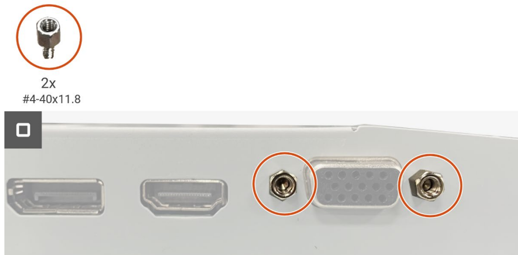
Figure 29. Installing the interface board
