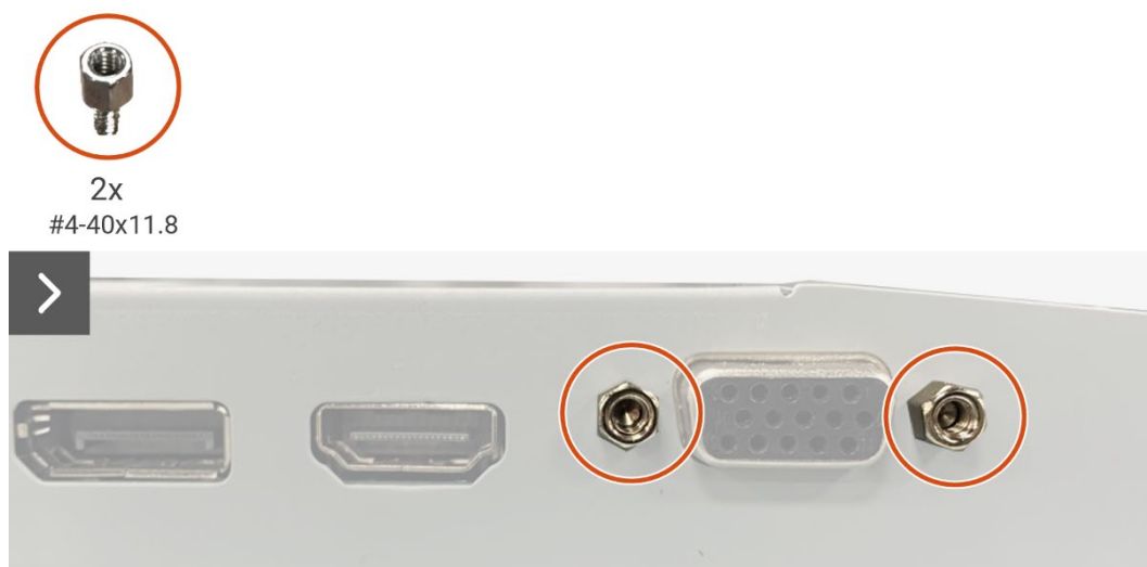
Figure 24. Removing the interface board
