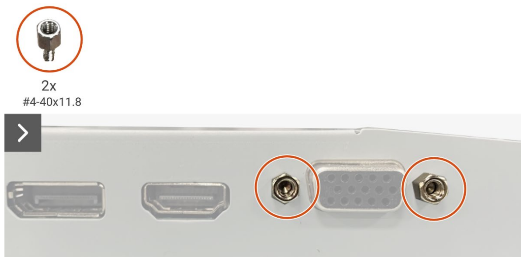
Figure 46. Removing the interface board
