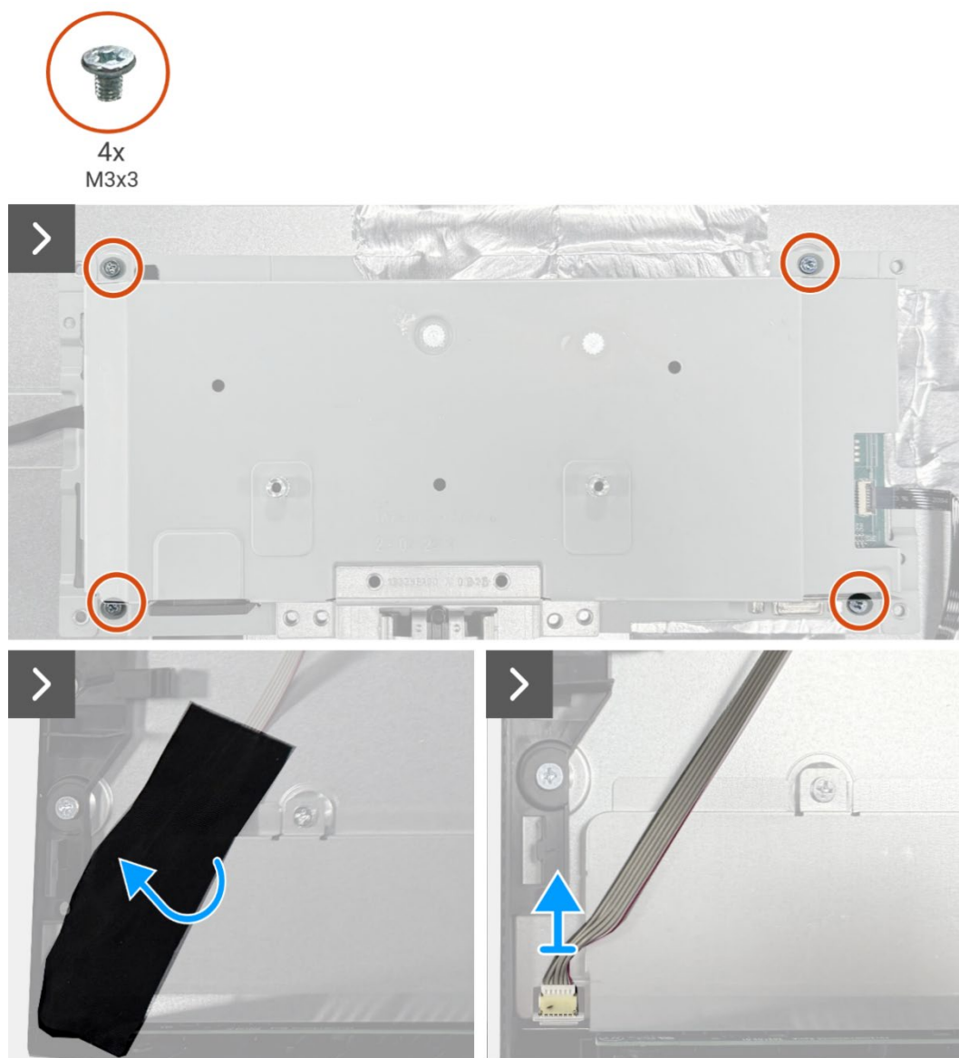
Figure 6. Removing the chassis assembly
