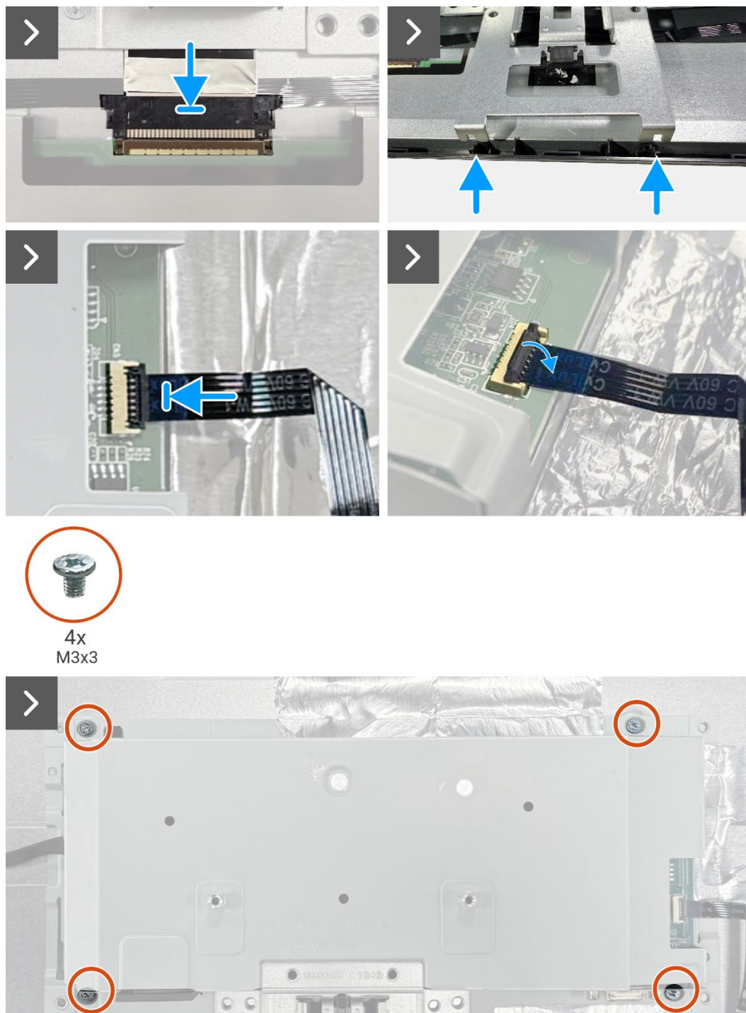
Figure 8. Installing the chassis assembly
