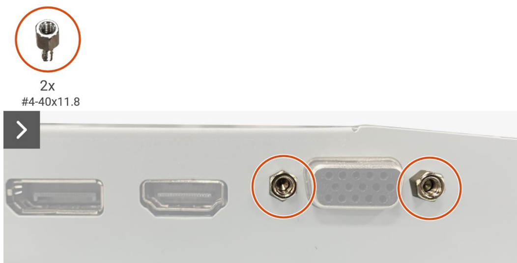
Figure 22. Removing the interface board
