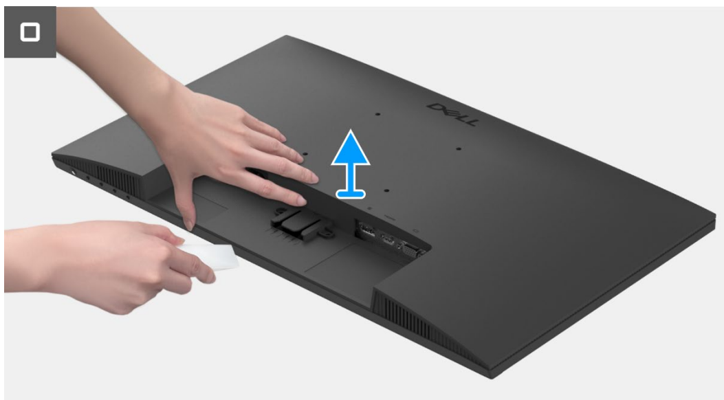
Figure 14. Removing the back cover
