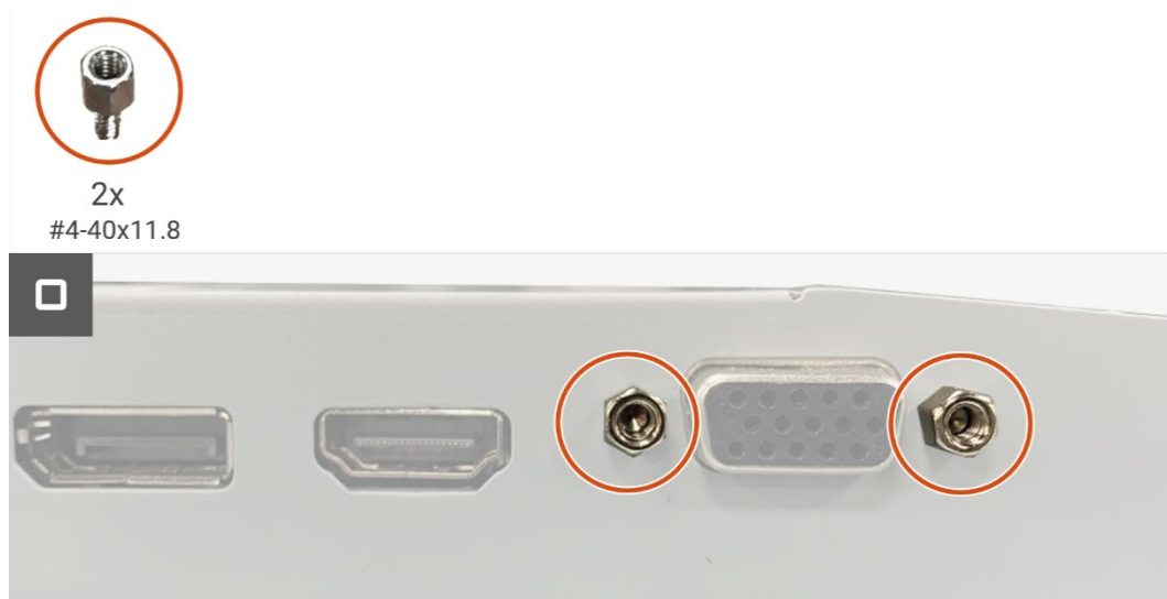
Figure 27. Installing the interface board
