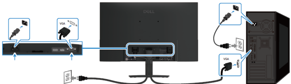
Figure 8. Connecting VGA cable
