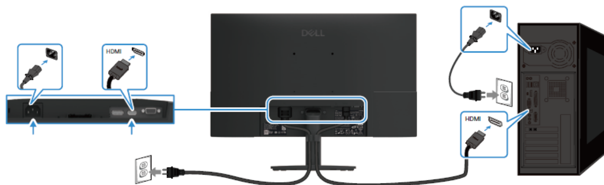
Figure 10. Connecting HDMI cable
