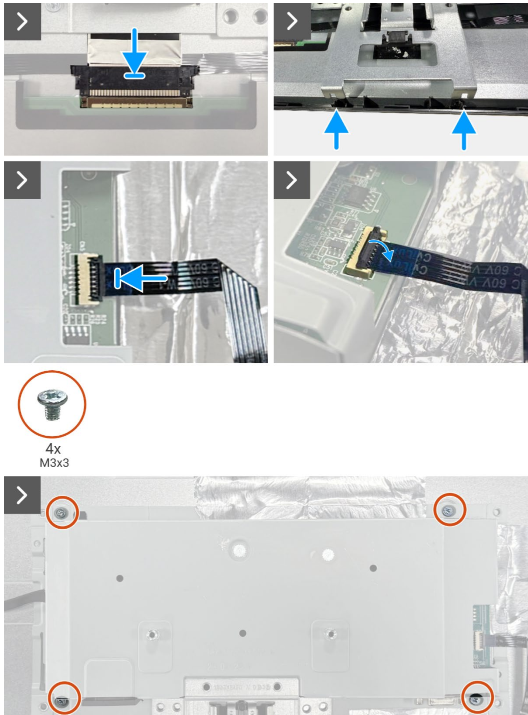
Figure 18. Installing the chassis assembly
