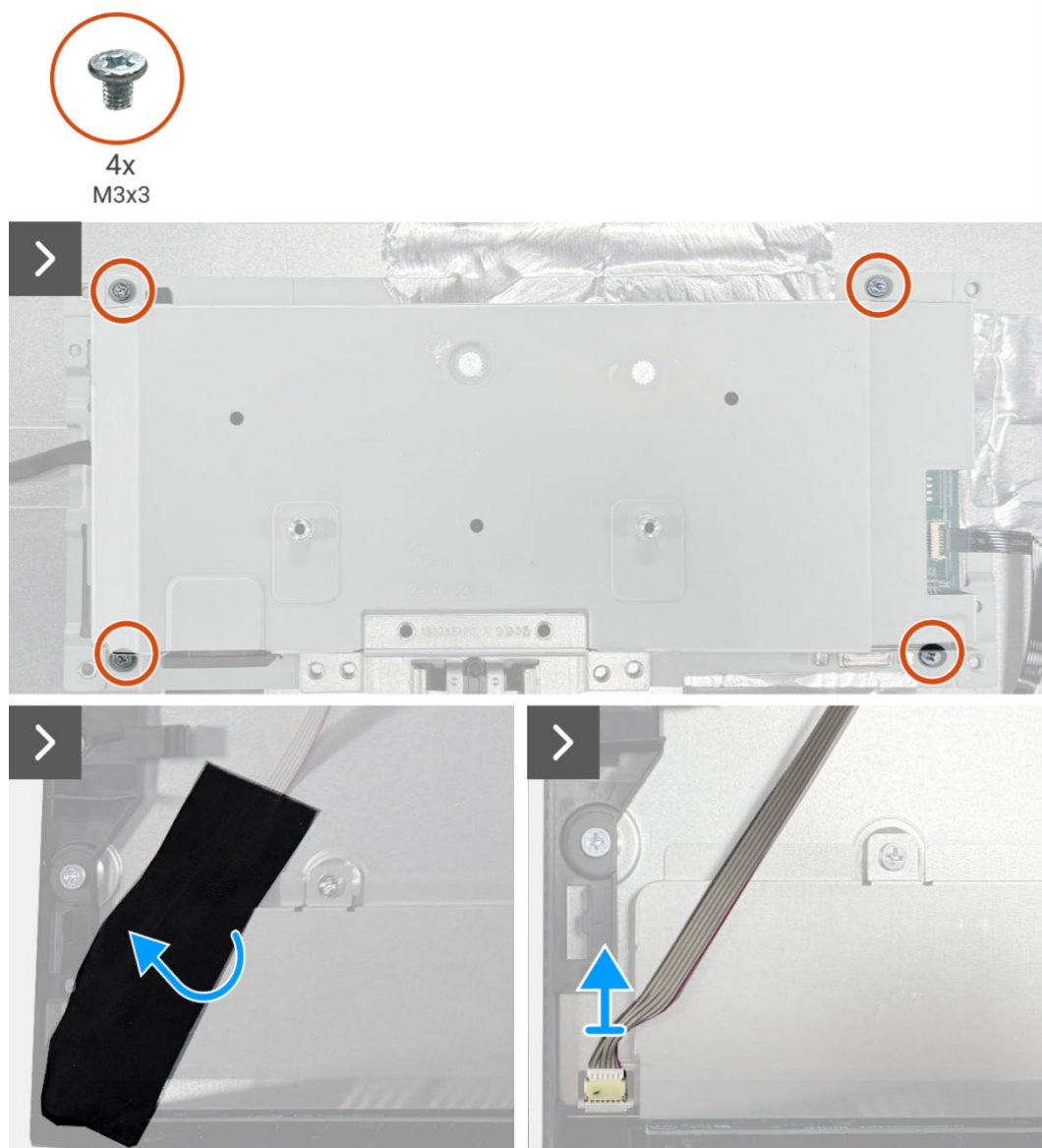
Figure 16. Removing the chassis assembly
