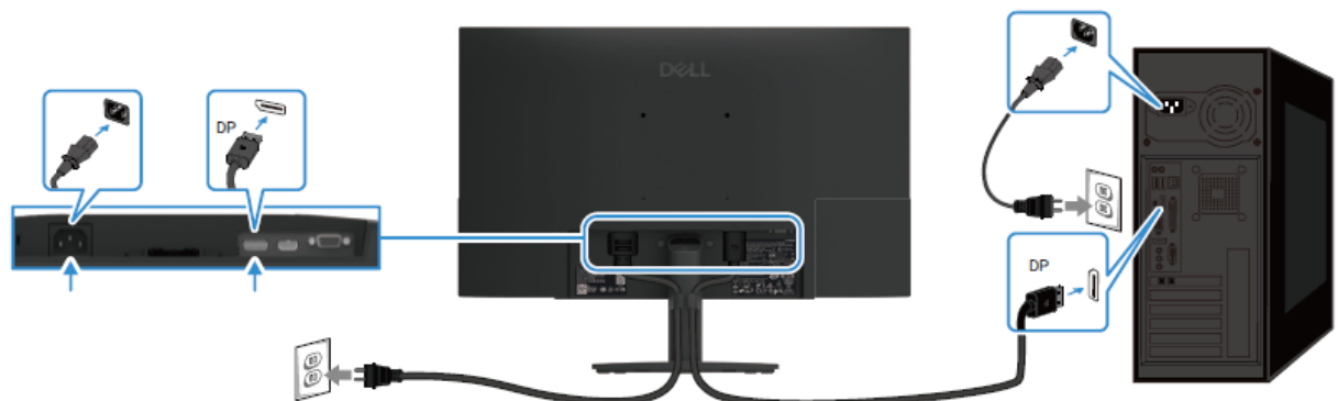
Figure 9. Connecting DP cable
