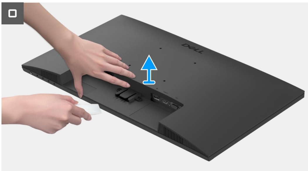
Figura 4. Remover a tampa traseira
