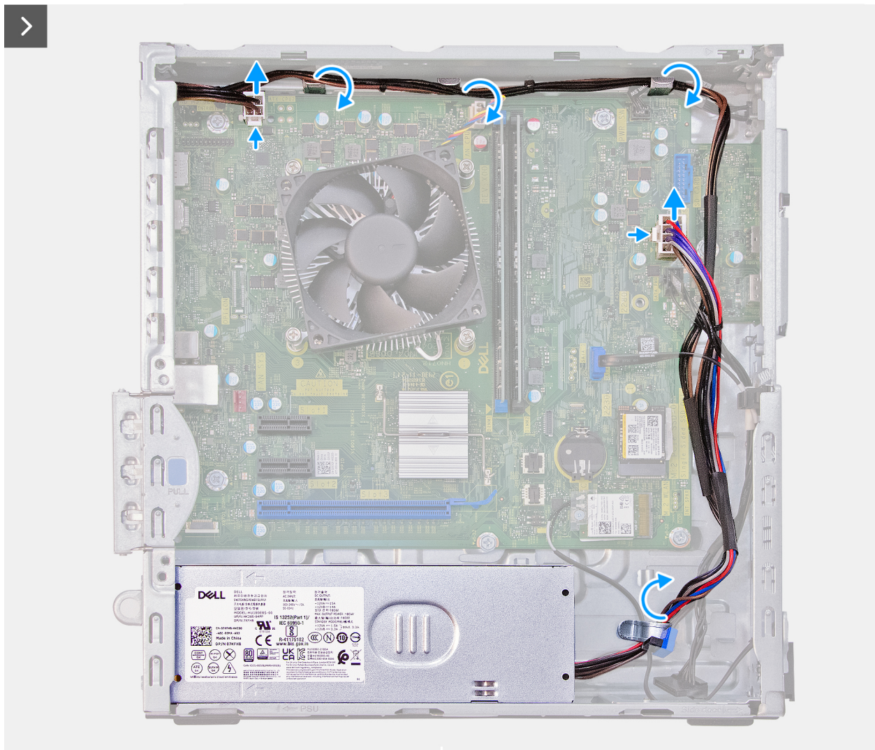
Figure 33. Removing the power-supply unit
