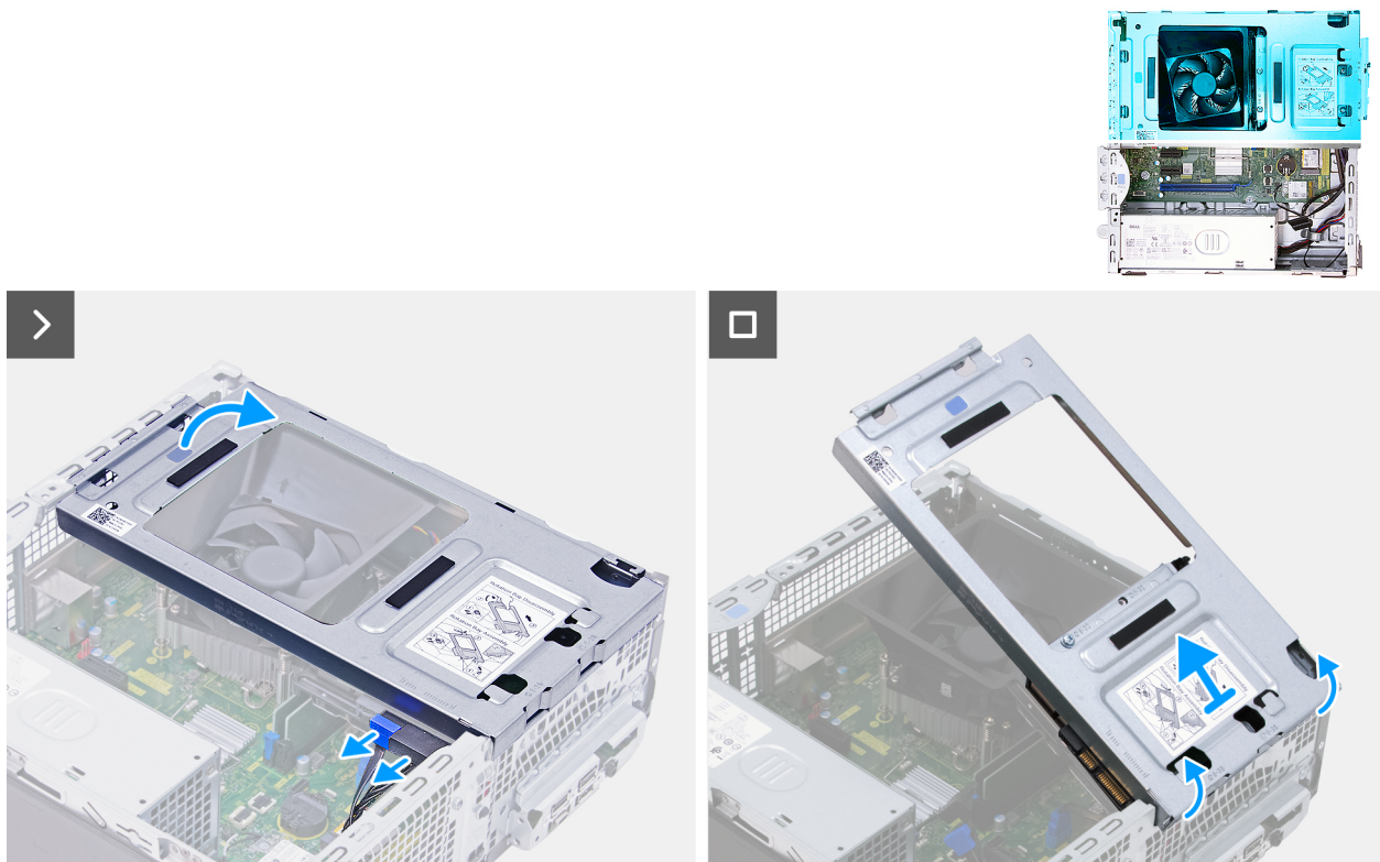
Figure 19. Removing the rotation bay
