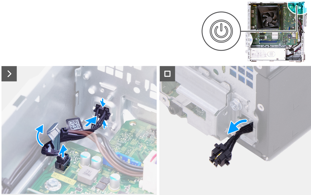
Figure 43. Removing the power button
