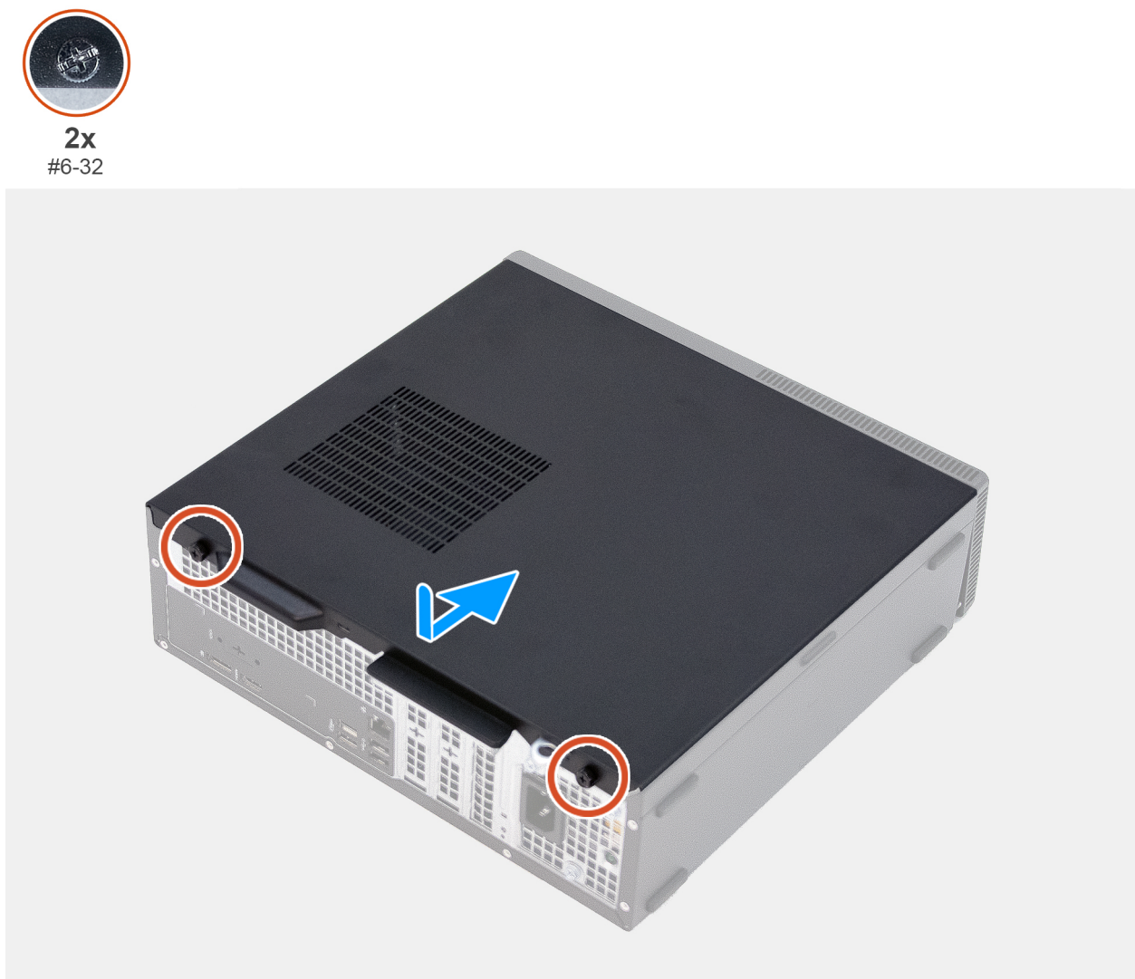
Figure 12. Installing the left-side cover
