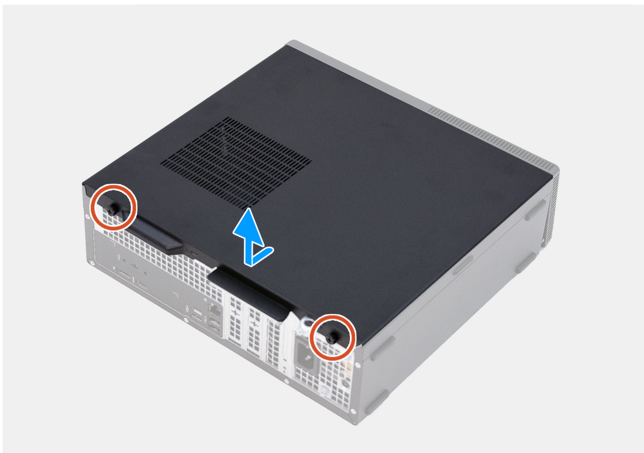
Figure 11. Removing the left-side cover
