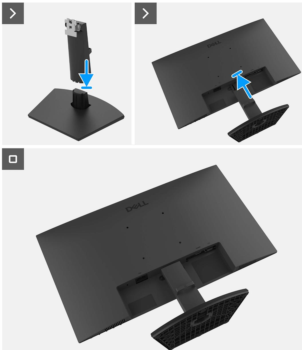
**Figure 11.** Installation du support
