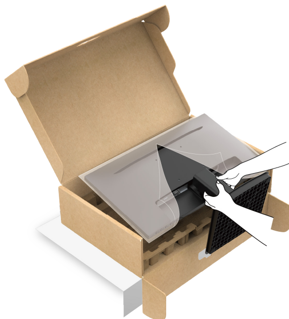
Figure 13. Hold the stand riser and lift the monitor
