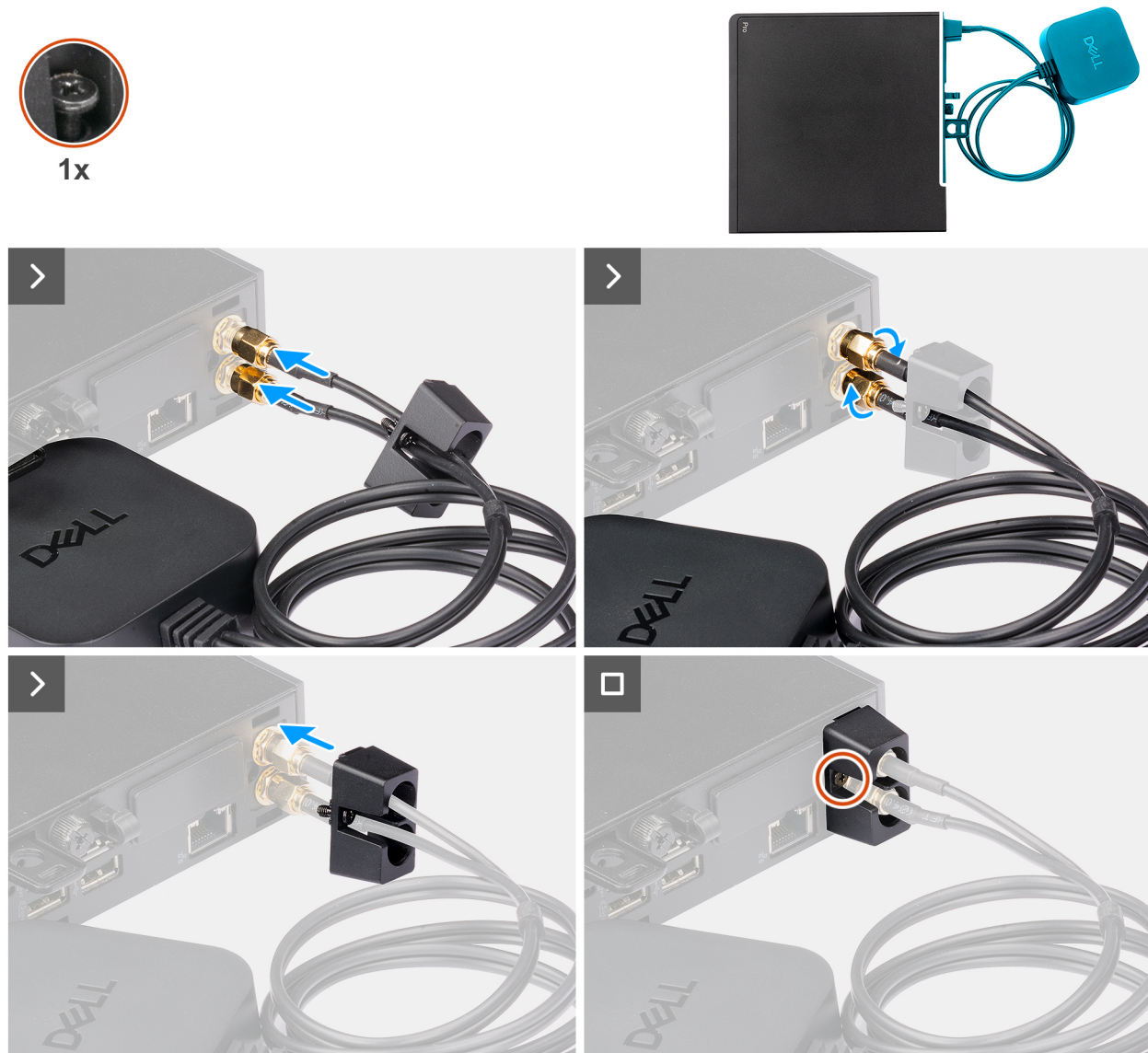
Figure 35. Installing external puck antenna
