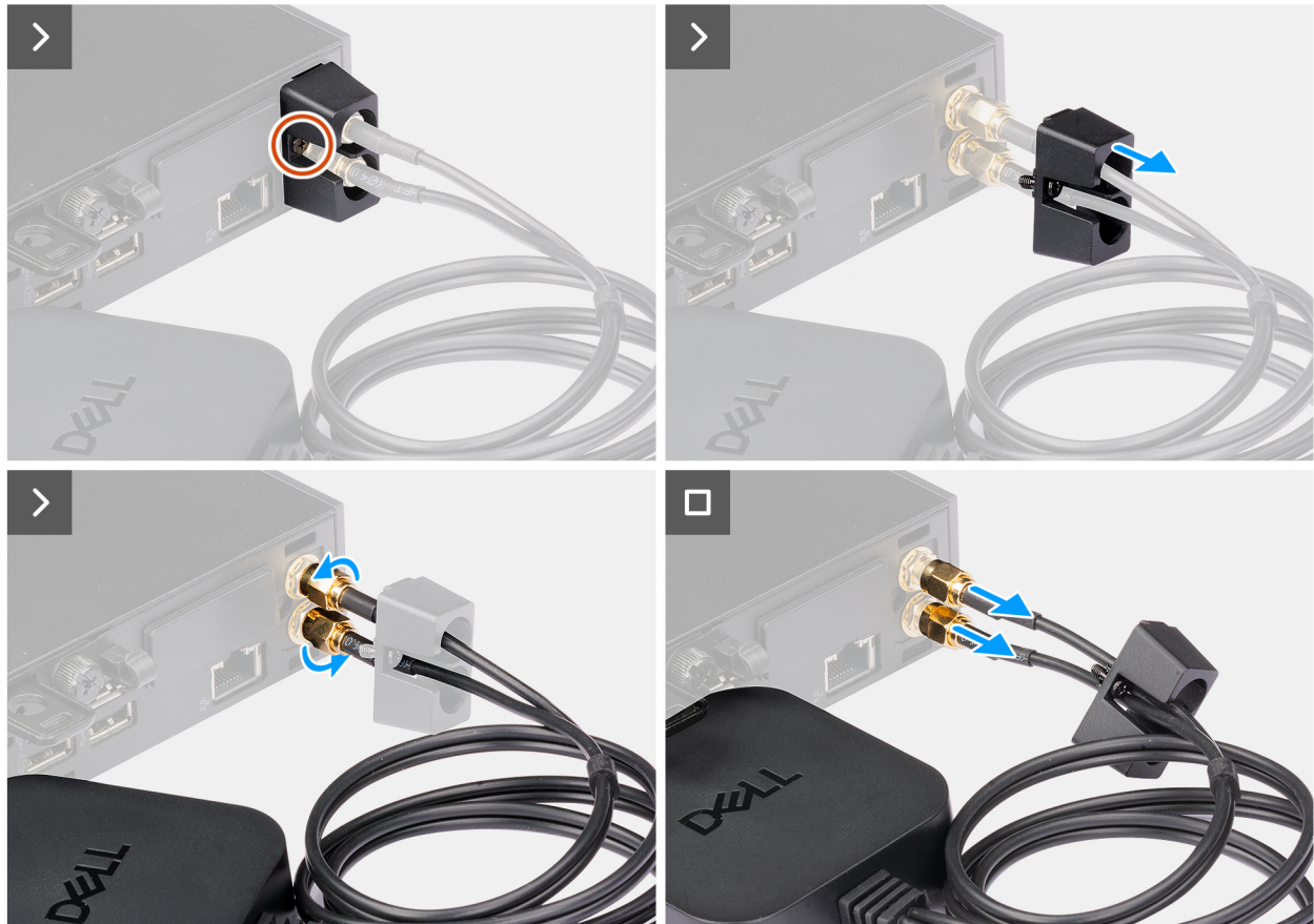
Figure 34. Removing external puck antenna
