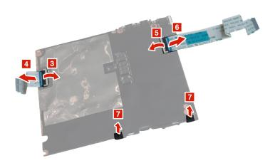
Figure 43. Disconnect the UB\_MB FFC and remove the microphone rubbers
