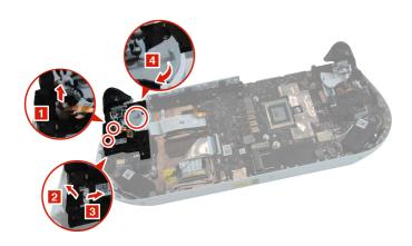
Figure 15. Disconnect the SWT PCB cable and disconnect the back key FPC
