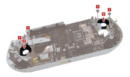
Figure 34. Remove screws and remove RGB lights
