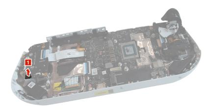
Figure 19. Remove the right motor
