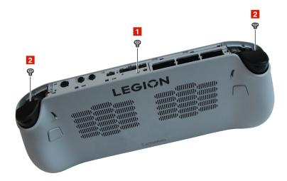
Figure 7. Remove screws at the top
