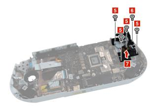
Figure 22. Remove screws and remove the left trigger button frame
