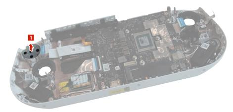
Figure 30. Remove the ABXY rubber
