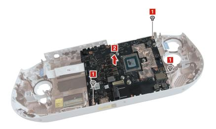
Figure 42. Remove screws and remove the system board
