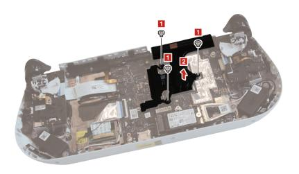
Figure 12. Remove screws and remove the heat sink
