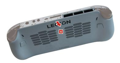
Figure 9. Remove the B cover
