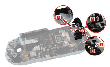
Figure 21. Disconnect the SWT PCB cable and disconnect the back key FPC
