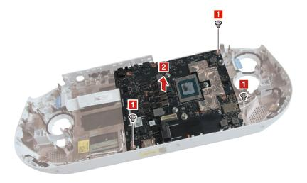
Figure 40. Remove screws and take the system board out
