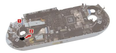
Figure 33. Remove one screw and remove the touchpad module
