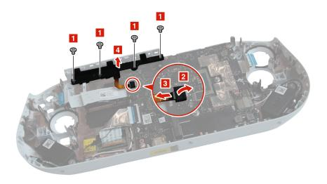
Figure 35. Remove screws, disconnect the ALS FPC, and remove the volume button bezel
