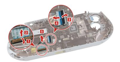
Figure 39. Disconnect the EDP cable and remove the EDP cable
