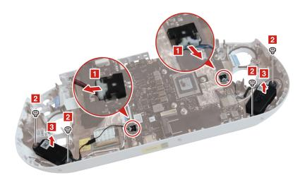
Figure 37. Disconnect speaker cables, remove screws, and remove speakers
