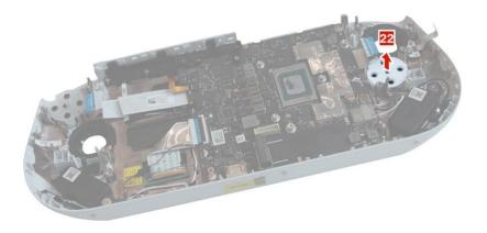
Figure 28. Remove the D-pad rubber
