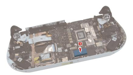
Figure 14. Remove the SSD pad
