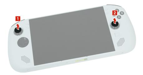
Figure 4. Remove the joystick caps
