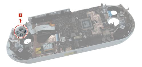
Figure 31. Remove the ABXY buttons
