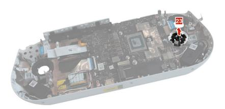
Figure 29. Remove the D-pad frame and D-pad button
