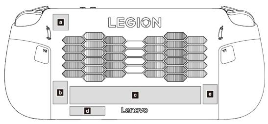
Figure 44. Label layout on the B cover
