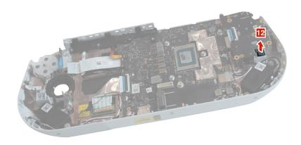
Figure 25. Remove the left motor
