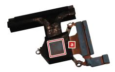
Figure 2. Areas on the heat sink where thermal interface materials should be applied
