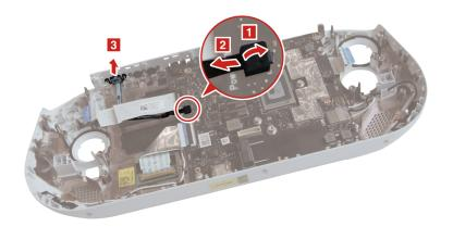
Figure 38. Disconnect the power button FPC and remove the power button
