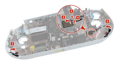
Figure 41. Tear the WiFi mylar, disconnect antenna cables, and tear antennas
