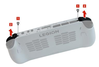
Figure 6. Remove screws and remove bumper buttons
