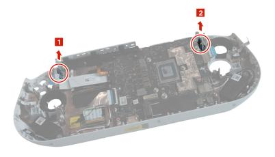
Figure 32. Remove the function buttons
