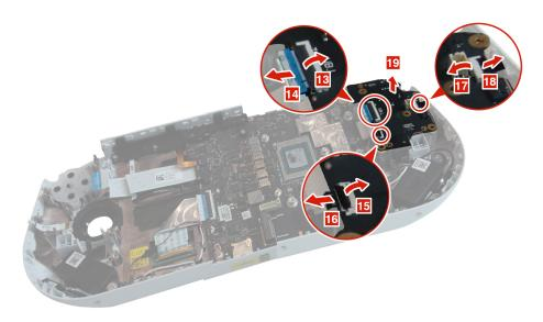
Figure 26. Disconnect the UB\_Ring FPC, disconnect the MB\_UB FFC, disconnect the D-pad board FFC, and remove the left board
