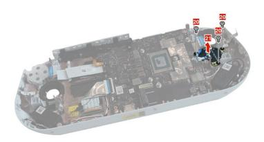
Figure 27. Remove screws and the D-pad board
