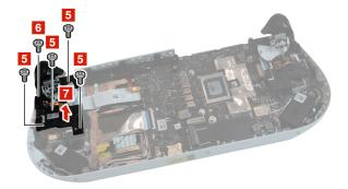
Figure 16. Remove screws and remove the right trigger button frame
