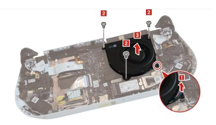
Figure 11. Disconnect the fan cable, remove screws, and remove the fan
