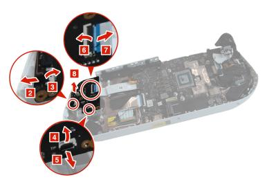
Figure 20. Disconnect the UB\_Ring FPC, disconnect the MB\_UB FFC, disconnect the touchpad board cable, and remove the right board
