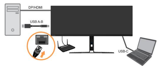
This monitor can support one PC to access internet stably by the Ethernet port with 2.5G bandwidth, thru USB-B port of monitor by USB A-B cable, or thru USB-C port.
