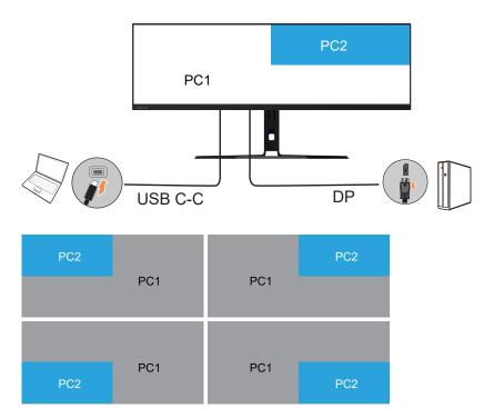
As same to PBP, the PIP (Picture-in-Picture) function can receive two different video sources too. The best resolution of foreground PC2 is 5120x1440@165Hz.
