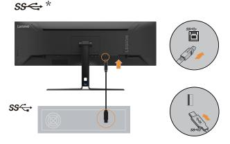
7. Connect one end of the USB cable to the USB downstream terminal on the side of the monitor, and connect the other end of the USB cable to an appropriate USB port on your device.
