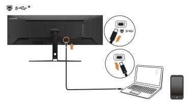
Note: The USB Type-C port of this monitor provides data, video and power transmission. The host device must support DisplayPort Alt mode (video, charging and USB 3.1) via the USB Type-C interface.
