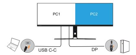
The PBP (Picture-by-Picture) function make the monitor to display two different video sources simultaneously. User can select any one of 4 inputs (DP, HDMI1, HDMI2, USB-C) for the left screen, select another input for the right one.
