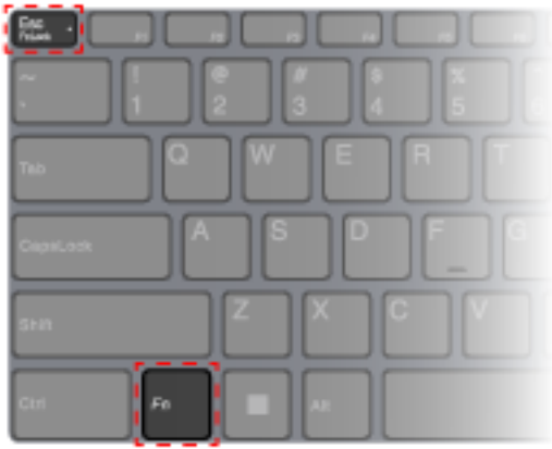
Figure 11. Locations of the FnLock key and the Fn key
