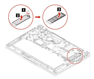
Step 2. Install the M.2 solid-state drive and its bracket in reverse order.
