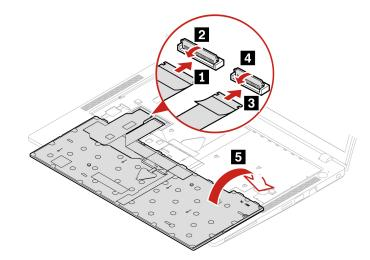
Step 2. Insert the keyboard into the keyboard bezel as shown. Ensure that the top edge of the keyboard (the edge that is close to the display) is under the keyboard bezel.
