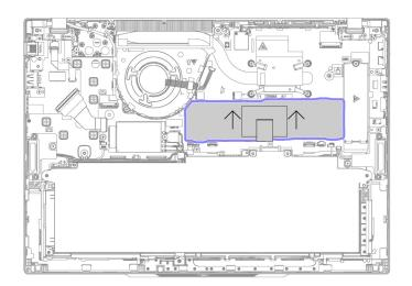
Step 1. Remove the memory module shielding cap as shown below. ThinkPad T14 Gen 6 / ThinkPad P14s Gen 6 AMD
