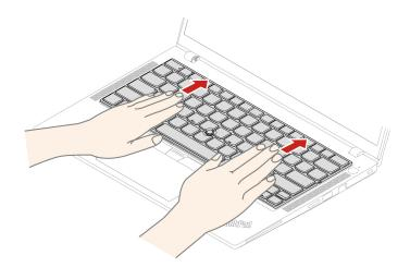
Step 3. Pivot the keyboard slightly upward **II** and then turn over the keyboard **II**.
