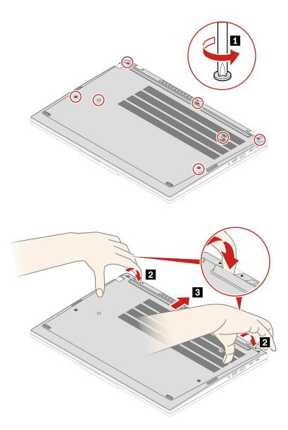
Step 2. Install the base cover assembly as shown below. ThinkPad T14 Gen 6 / ThinkPad P14s Gen 6 AMD
