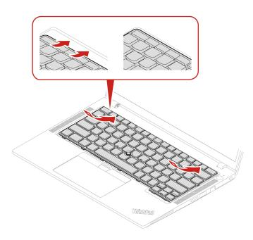
Step 3. Slide the keyboard in the direction as shown. Ensure that the latches are secured under the keyboard frame.
