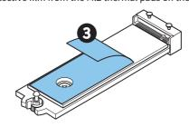
If you install 2260 SSD, use the included EZ M.2 Clip II Remover. Remove the plate screw and install EZ M.2 Clip II in the slot by using the remover. Skip this step if you install 2280 SSD.
