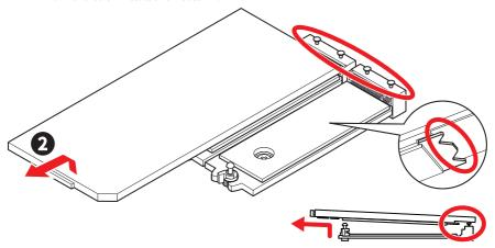
3. Remove the protective film from the M.2 thermal pads on the M.2 plate.
