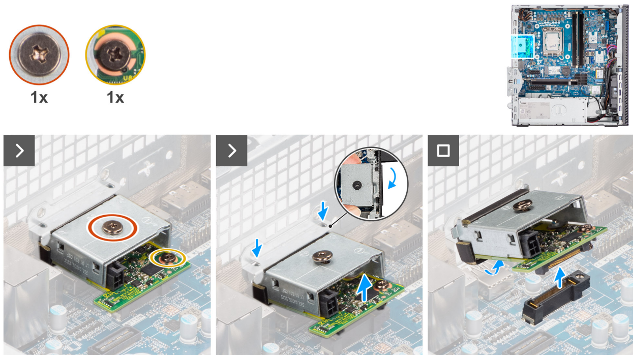
Figure 67. Removing the optional Thunderbolt module
