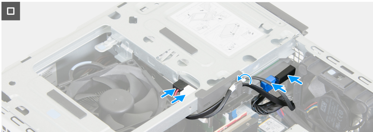
Figure 24. Installing the drive bay
