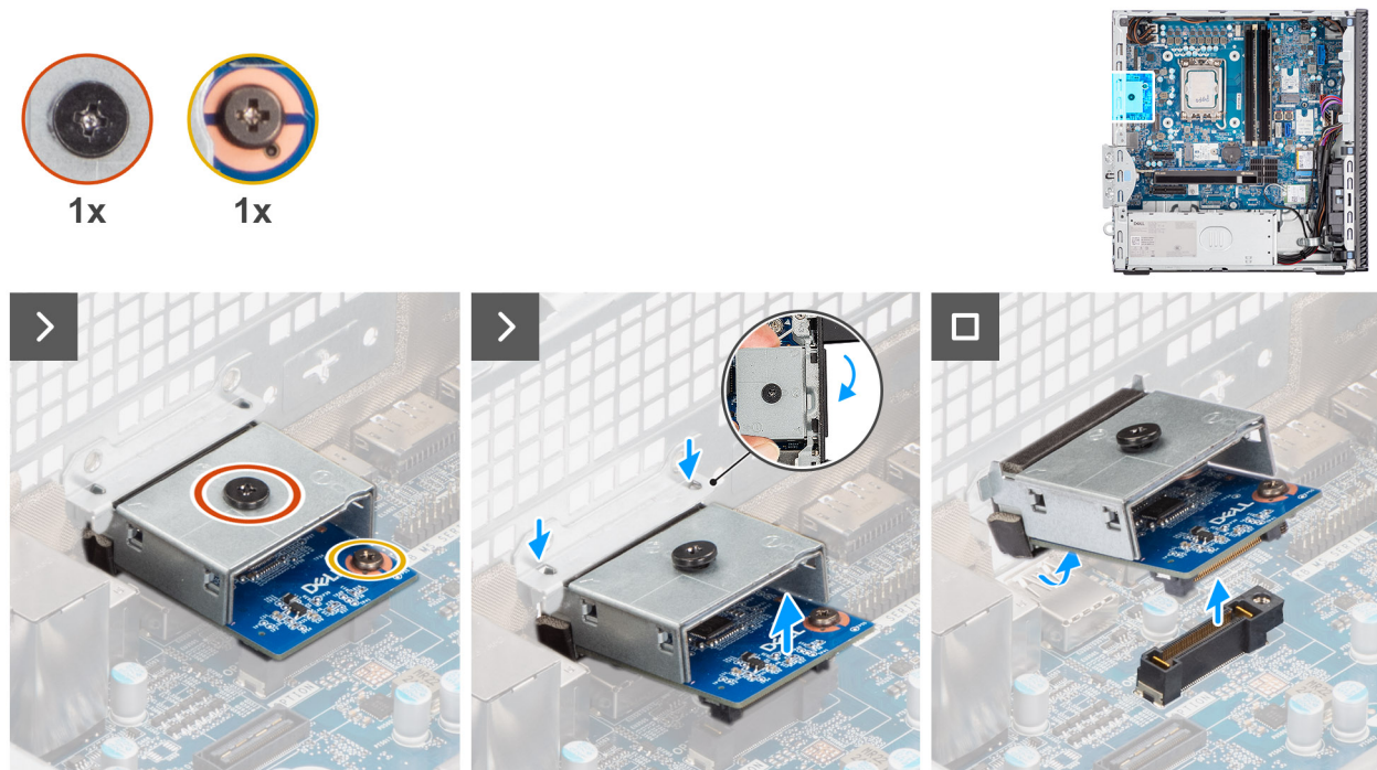
Figure 73. Removing the optional HDMI module
