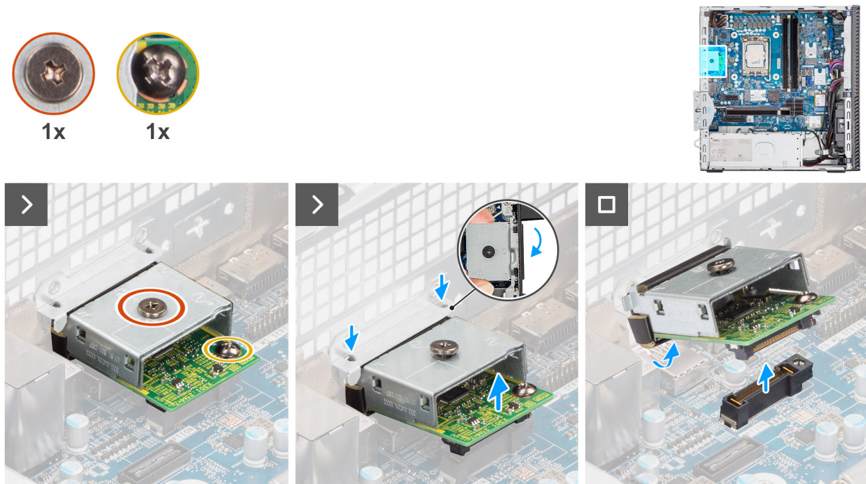
Figure 76. Removing the optional DisplayPort module
