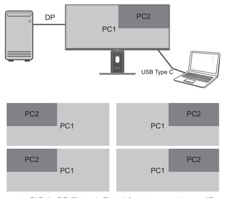
As same to PbP, the PiP (Picture-in-Picture) function can receive two different video sources too.
