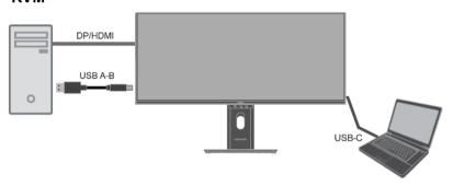
Step 2 The shortcut key of KVM on right direction of five-way key. The USB devices will be switched to another upstream port after OSD disappears. Note: KVM operation may cause USB device to be interrupted.
