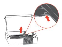
Step 3: Remove the base and stand from the monitor, refer to "Detaching the monitor base and stand" on page 2-12.
