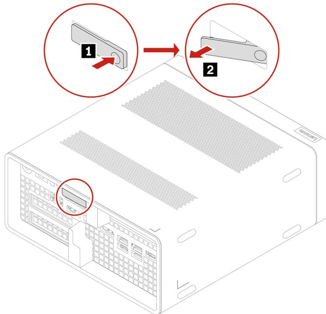
2. Pull the latch to remove the chassis.
