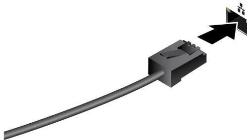
**Note:** For models with an Intel X710-T2L Ethernet adapter, it's recommended to prepare a Shielded Twisted Pair (STP) Category 6A Ethernet cable for Ethernet connection on the adapter.
