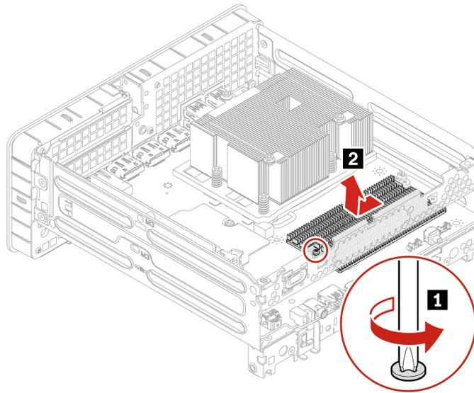
3. Remove the M.2 solid-state drive. Find screw specification in the following screw table.
