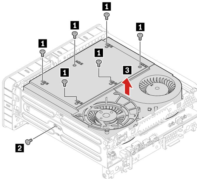
2. Remove the M.2 solid-state drive heatsink. Find screw specification in the following screw table.
