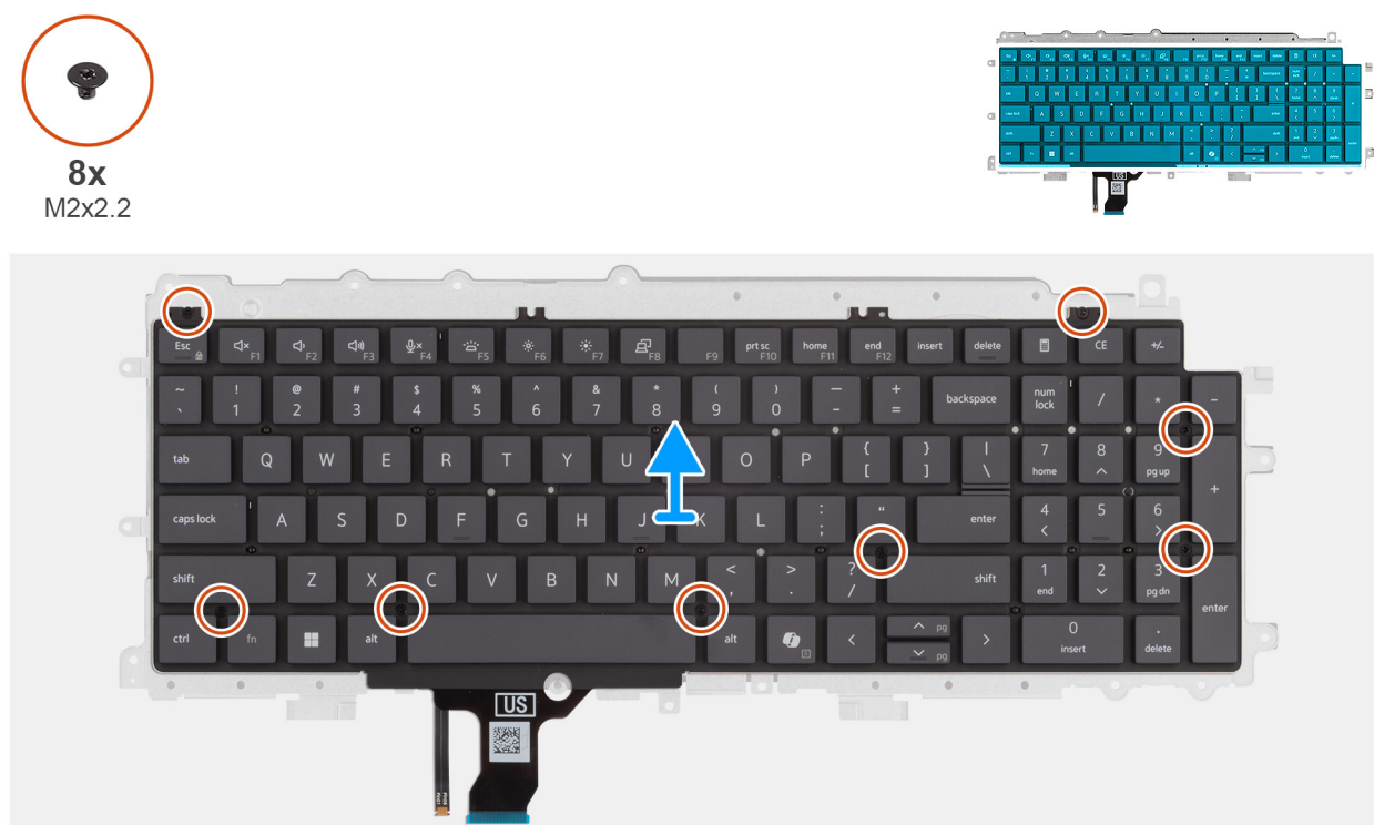
Rysunek 56. Removing the keyboard support plate
