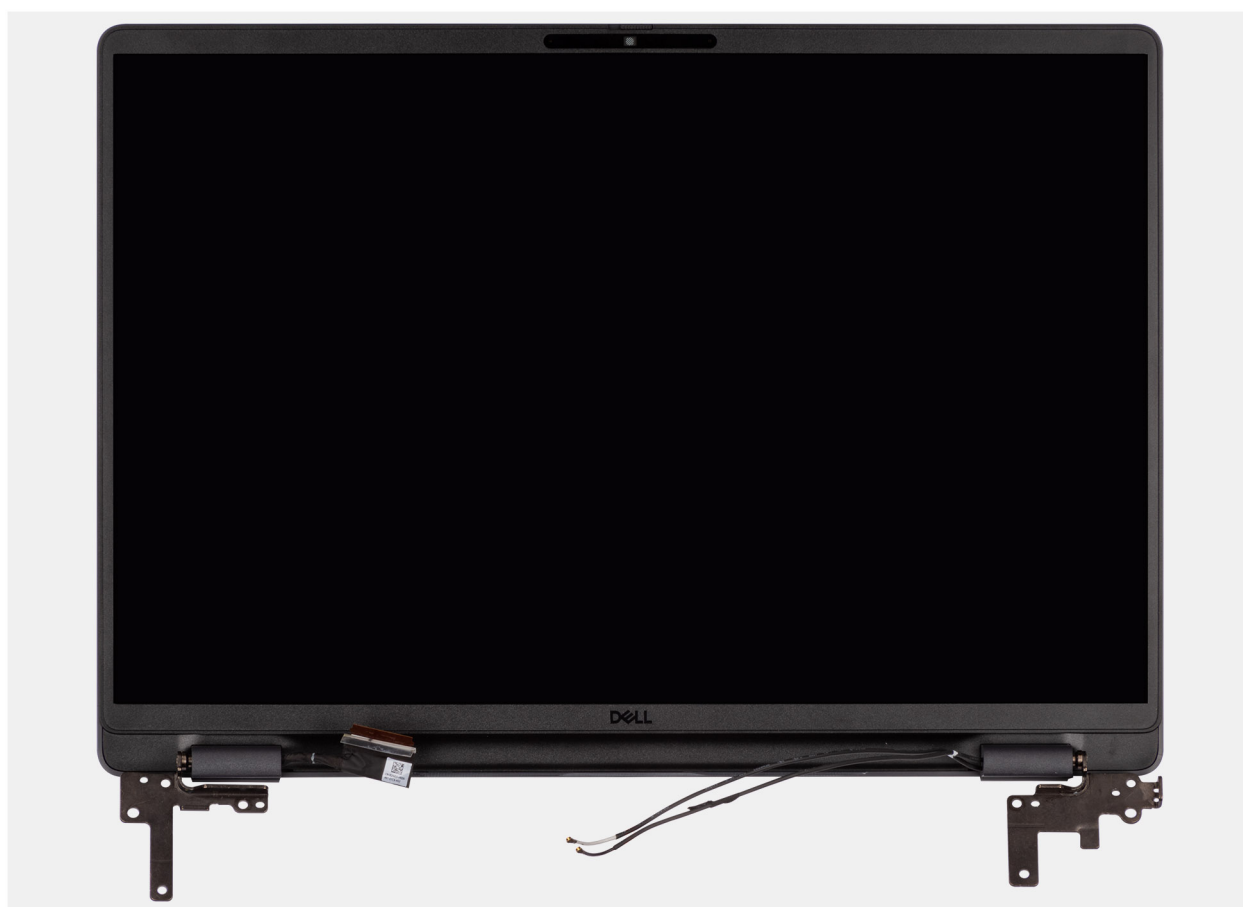
Rysunek 64. Removing the display assembly
