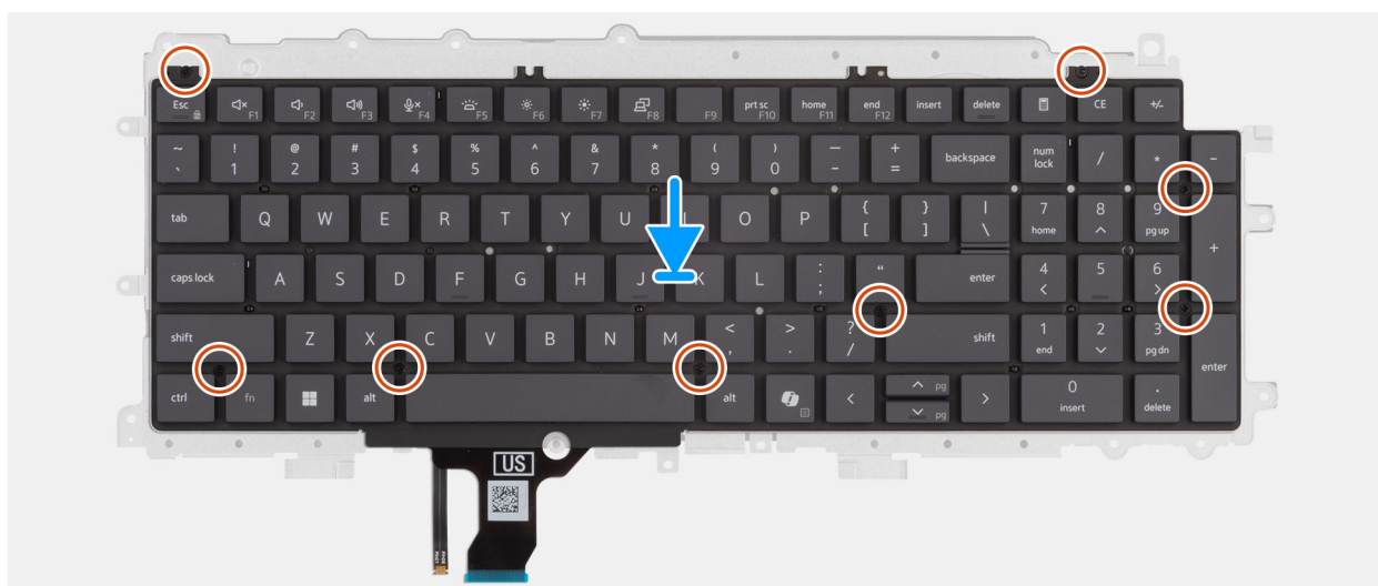
Rysunek 59. Installing the keyboard support plate
