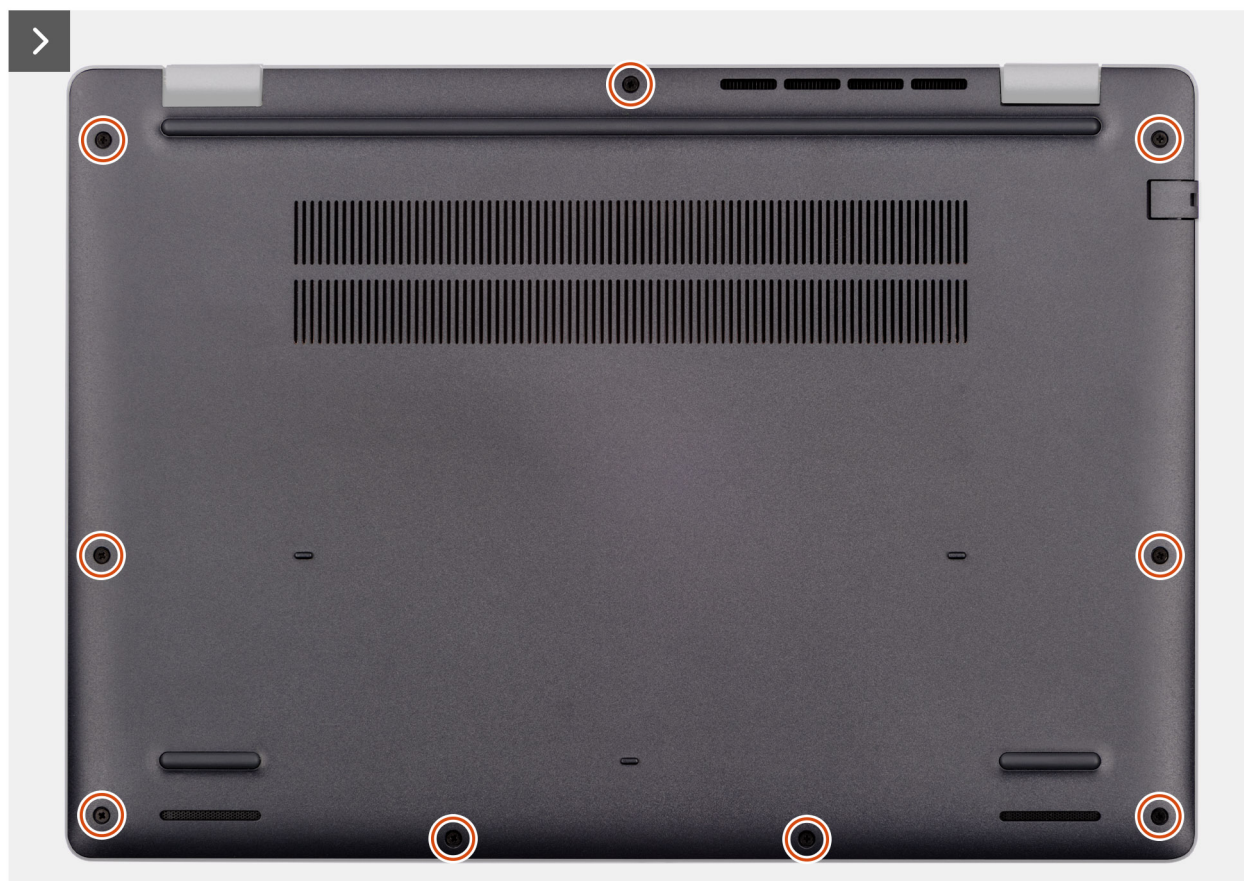
Rysunek 11. Removing the base cover
