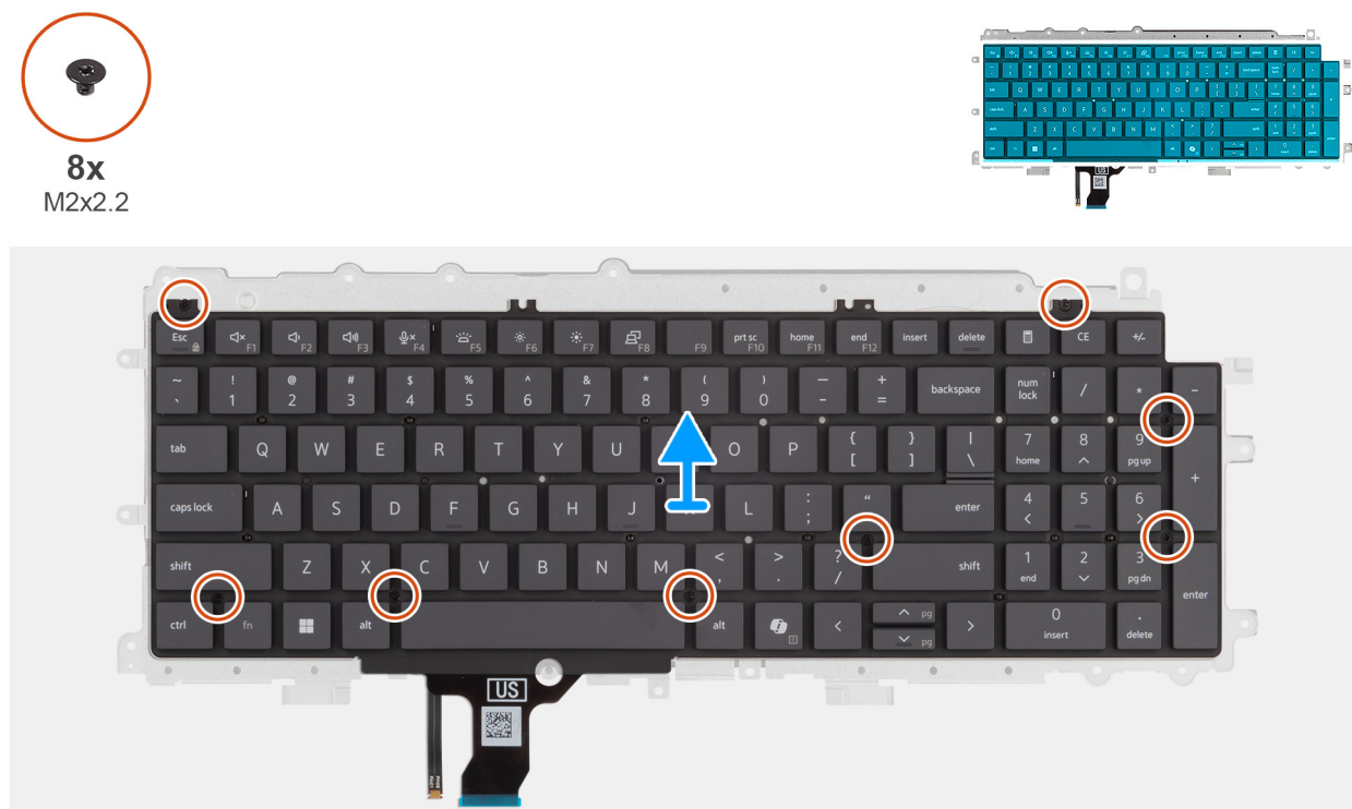
Rysunek 66. Removing the keyboard support plate
