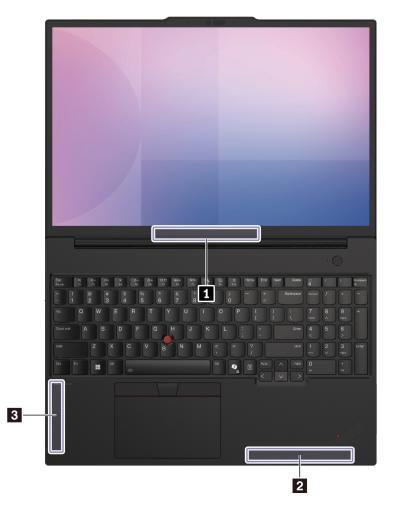
Wireless LAN combo antenna (main and auxiliary)
