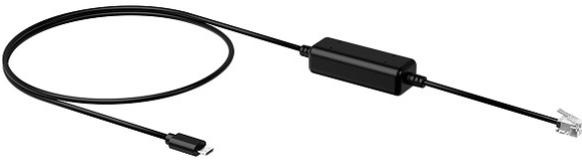
The unit is easy to install; simply link EHS35 to the RJ9 (4P4C) headset port of the phone. Its plug-and-play effectively gives you the ability to remotely control your Yealink phone calls, including answering, rejecting, holding, muting, hanging up, switching between multiple calls, and adjusting the volume.
