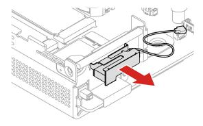
2. Align the two feet of the front Wi-Fi antenna with the two holes on the antenna bracket and install the front Wi-Fi antenna to the antenna bracket.
