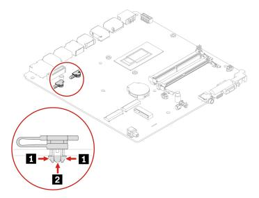
2. Insert a new M.2 SSD clip into the hole on the system board.
