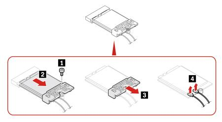
3. Install a new Wi-Fi card or Wi-Fi card shield in reverse order.
