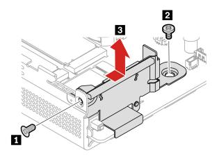
3. Install a new antenna bracket in reverse order.
