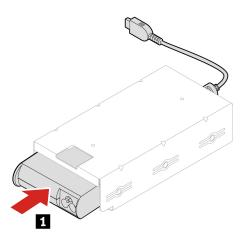
2. Connect the power cord to the ac power adapter.
