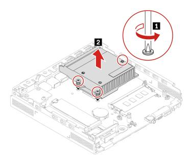
3. Install a new CPU heat sink in reverse order.
