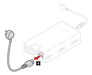
4. Push down the ac power adapter from the top hole of the power adapter bracket. Push the ac power adapter out of the power adapter bracket.
