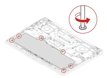
b. Remove the battery as shown below.
