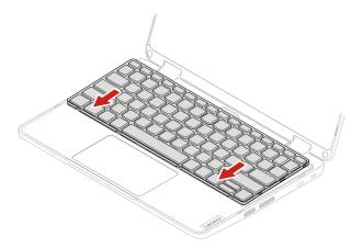
Step 3. Slightly push the keyboard as shown and ensure that it is seated correctly.
