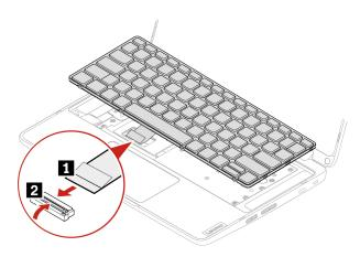
Step 2. Insert the keyboard into the keyboard bezel as shown. Ensure that the bottom edge of the keyboard (the edge that is close to the trackpad) is under the keyboard bezel.
