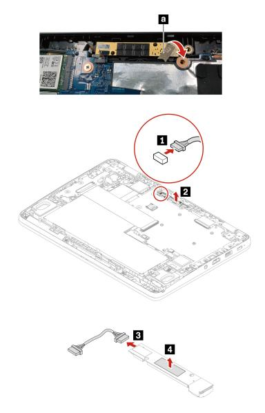
Install the camera, camera cable, and sponge in reverse order. After installing: attach the conductive tape 🔳 to the camera as shown. Do not touch the other end of the conductive tape.
