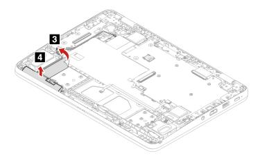
Step 2. Install the main wireless WAN antenna in reverse order. When installing, ensure that the connector is attached firmly.
