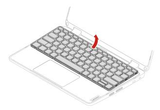
Step 5. Detach the connector and remove the keyboard.
