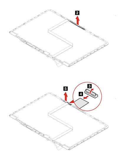
Step 2. Install the camera-and-microphone board and sensor board in reverse order.
