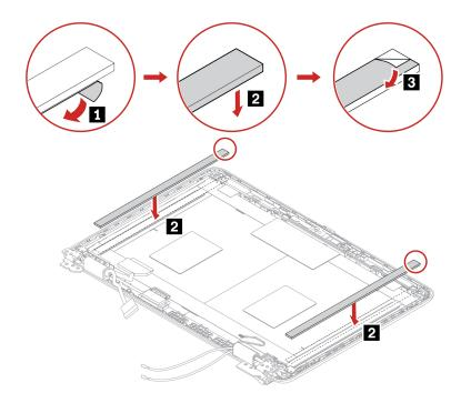
Step 2. Attach the LCD cable to the LCD module assembly as shown. Turn over the LCD module assembly to secure the LCD module assembly with tapes.
