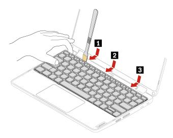
Step 4. Pivot the keyboard slightly upward.
