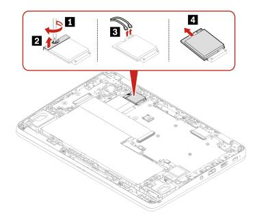
Step 2. When installing: Plug the gray cable into the main connector, and the black cable into the auxiliary connector on the module.
