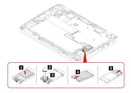
Step 2. Install the M.2 solid-state drive and its bracket in reverse order.
