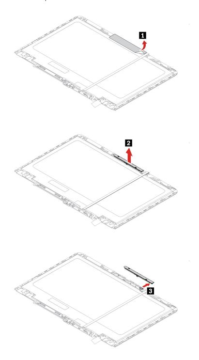
Step 2. Remove the sensor board as shown below.
