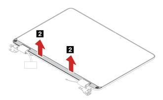
Step 2. Install the strip cover caps and strip cover in reverse order. When installing, ensure that all the latches are attached firmly.
