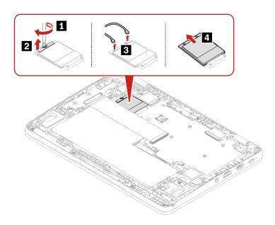
Step 2. Install the wireless WAN module and its bracket in reverse order.
