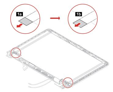
Step 2. Turn over the LCD module assembly and detach the LCD cable from the LCD module assembly as shown.
