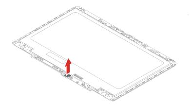
Step 3. Install the camera-and-microphone board and sensor board in reverse order.
