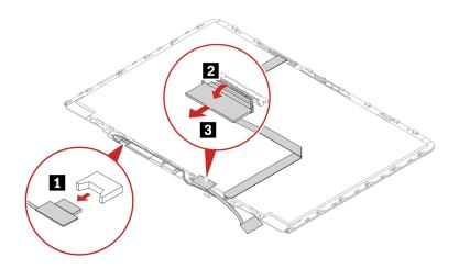
Step 2. Install the LCD cable in reverse order.
