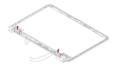
Step 2. Install the LCD hinge caps in reverse order.
