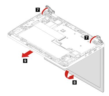
Step 2. Install the LCD unit in reverse order.
