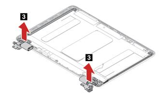
Step 2. Install the LCD hinges in reverse order.
