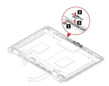
Step 2. Install the Webcam privacy shutter and camera-and-microphone board in reverse order.
