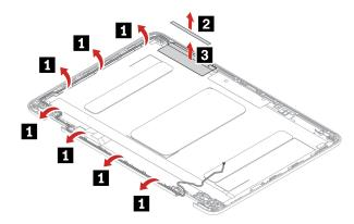
Step 2. Install the wireless WAN antenna assembly in reverse order.
