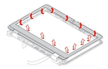
Step 2. Install the LCD bezel in reverse order. When installing, ensure that all the latches are attached firmly.
