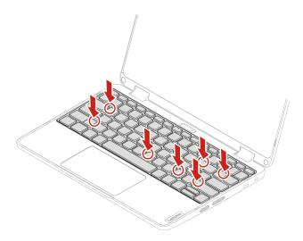
Step 4. Tighten the screw to secure the keyboard.
