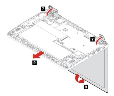
Step 2. Install the LCD unit in reverse order.
