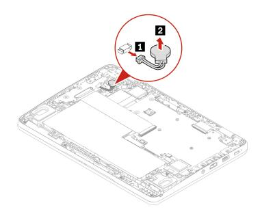
Step 2. Install the coin-cell battery in reverse order.
