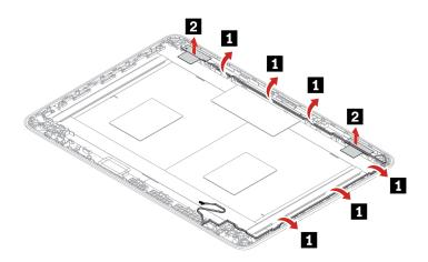
Attention: When you route the cables, ensure that they are not subject to any tension. Tension could cause the cables to be damaged by the cable guides, or a wire to be broken.
