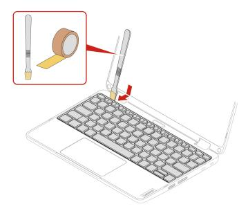
Step 3. Release the latches from the keyboard bezel assembly one by one in the direction as shown by arrows 1, 2, and 3, keep the top left corner of the keyboard in released position during the whole process.
