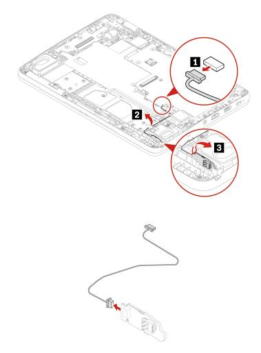
Step 2. Install the Lenovo Integrated Pen board and cable in reverse order.
