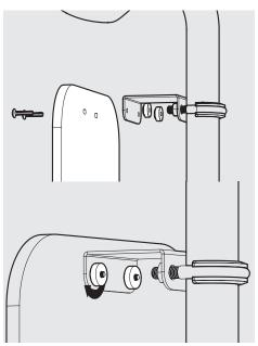
B5 Locate the Front Board to the Bracket Mount. Secure with the supplied Plastic Screws & Nuts.
