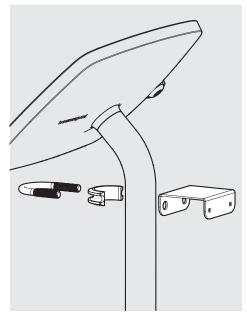
A2 Locate the top Bracket Mount & Mount Bolt to Floorstanding pole.
