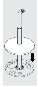
Orientate, locate & secure the Elevate Pole to the Base as shown. Ensure that all fixings are installed correctly.
