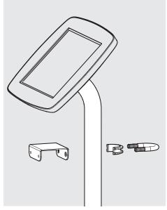
B2 Locate the top Bracket Mount & Mount Bolt to the Floorstanding pole.
