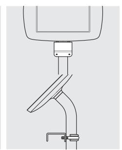
B3 Ensure the Bracket Mount & Mount Bolt are positioned correctly as shown.
