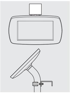
A3 Ensure that the Bracket Mount & Mount Bolt are positioned correctly as shown.
