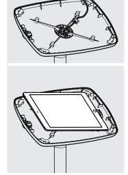
Install the Tablet into the 11 Case & connect to Power Cable.
