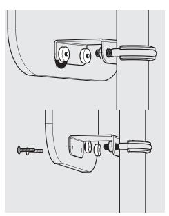
Secure the bottom section of the Front Board with the Plastic Screws & Nuts. Installation now complete.
