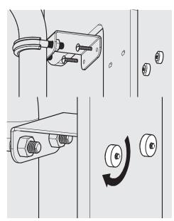
A5 Locate the Placard Board to the Bracket Mount. Secure with the supplied Plastic Screws & Nuts.
