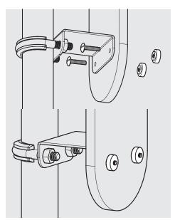
A7 Secure the bottom section of the Placard Board with the Plastic Screws & Nuts. Installation now complete.
