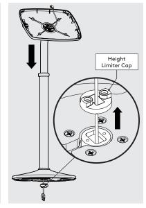
Feed the Power Cable through the Case, Elevate Pole & Height Limiter Cap.
