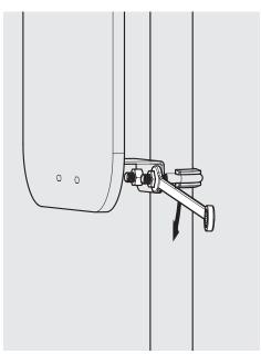
Locate & secure the bottom Bracket Mount & Mount Bolt. Tighten the nuts evenly.
