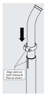
Reattach the Clamp without tightening.
