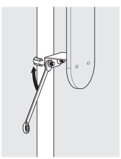
A6 Locate & secure the bottom Bracket
