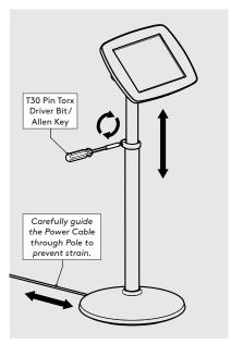
Adjust the Elevate Pole to your 13 desired height & tighten the Clamp.
