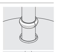
With the Cover on the 15 ground, locate & fit the Rubber Collar.
