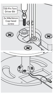
Attach the Height Limiter Cap to the Elevate Pole. Feed both Cables through the Base
