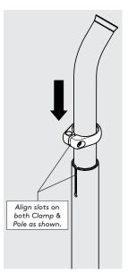
Reattach the Clamp without tightening.
