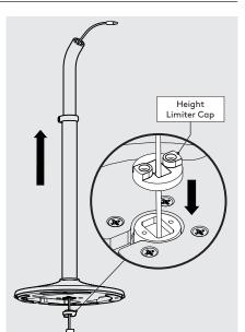
Feed the printer's power cable through the Height Limiter Cap & the Elevate Pole.
