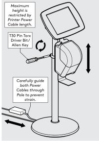
Adjust the Elevate Pole to your desired height & tighten the Clamp.
