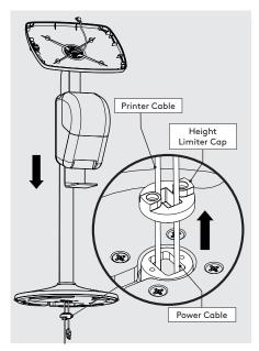
Feed the Power Cable through the Case, Elevate Pole & Height Limiter Cap.
