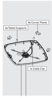
Install the Tablet Setup Kit. Each kit is specific per device & case.
