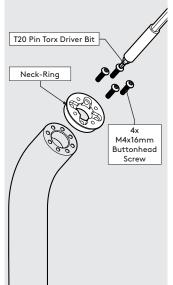
Remove Neck-Ring using T20 driver bit &
