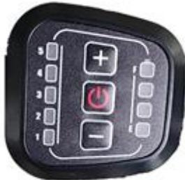
The bicycle is equipped with five levels of pedal assist, selectable on the display. The display is used to turn on the bicycle, view the remaining battery charge, and adjust the pedal assist.
