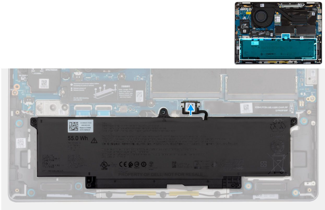
Figure 25. Connecting the battery cable
