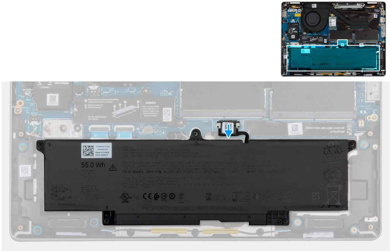
Figure 24. Disconnecting the battery cable
