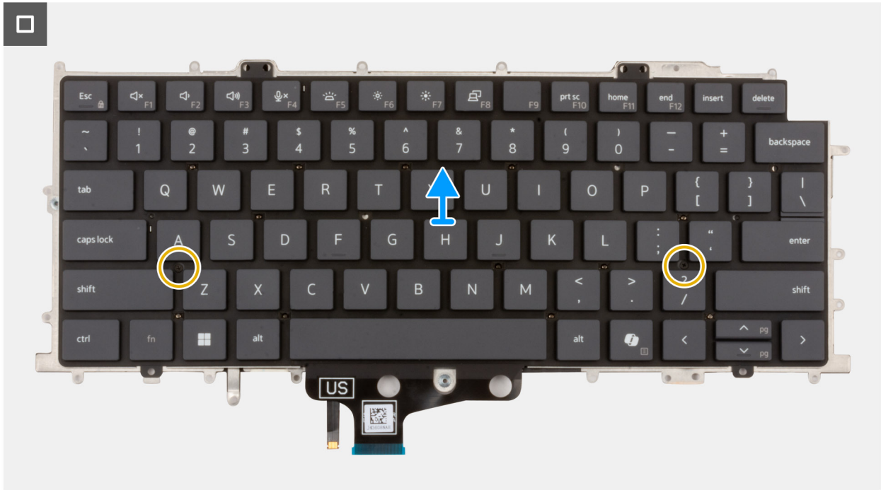
Figure 99. Removing the keyboard
