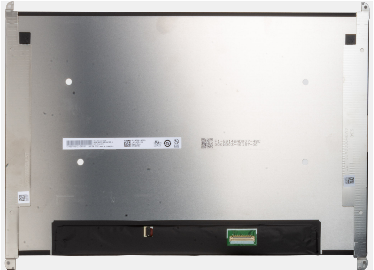
Figure 77. Display panel with brackets
