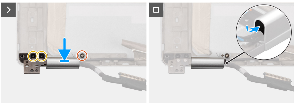
Figure 87. Installing the display cable
