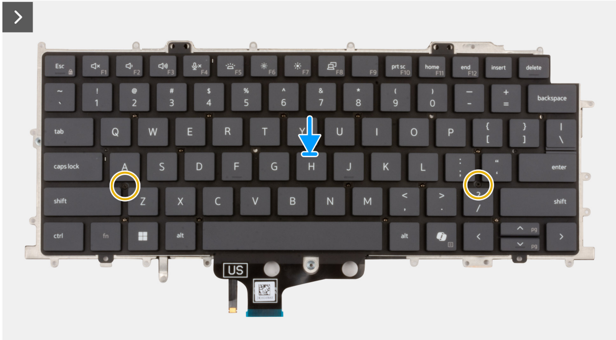
Figure 100. Installing the keyboard
