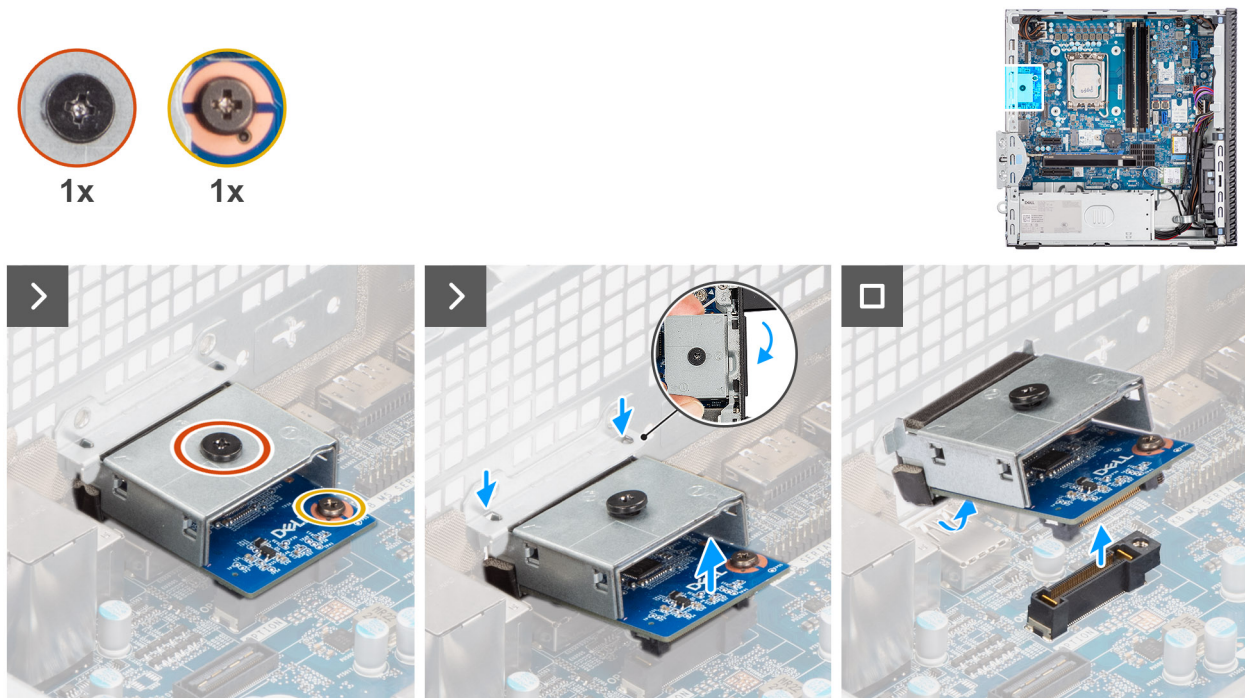
Figure 73. Removing the optional HDMI module
