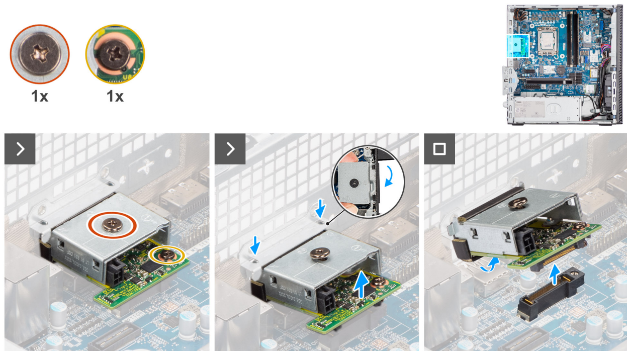
Figure 67. Removing the optional Thunderbolt module
