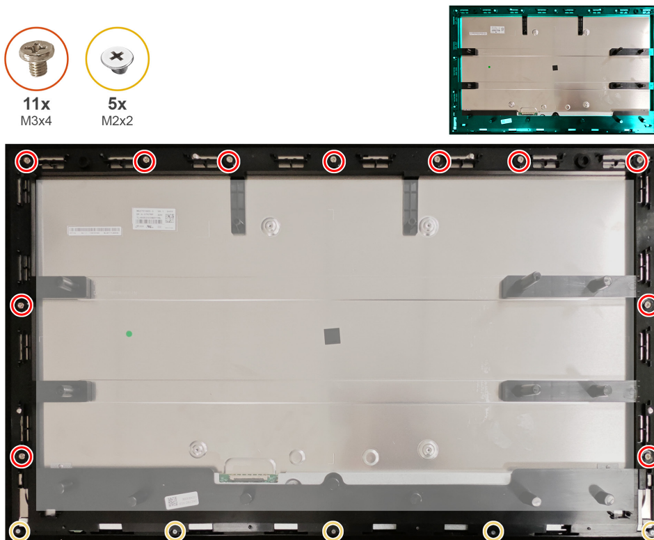
Figure 37. Installing the middle frame
