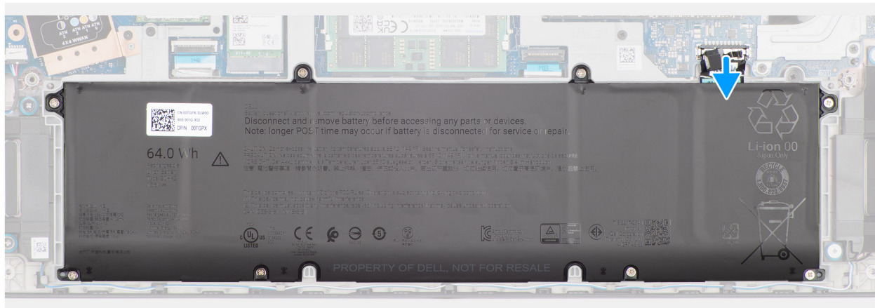
Figure 14. Removing the battery cable
