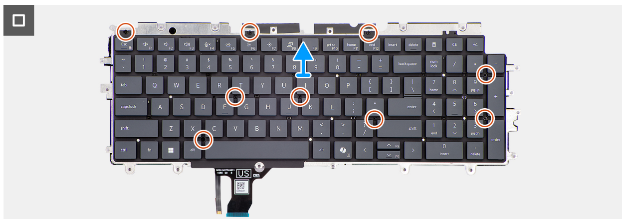
Figure 89. Removing the keyboard
