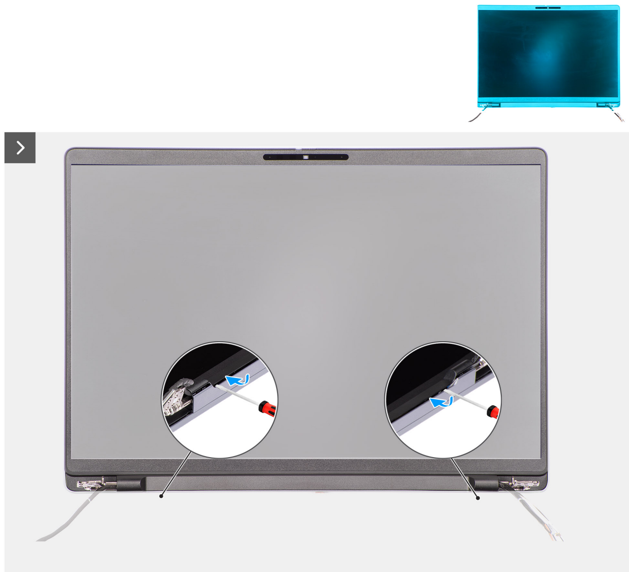
Figure 56. Removing the display bezel
