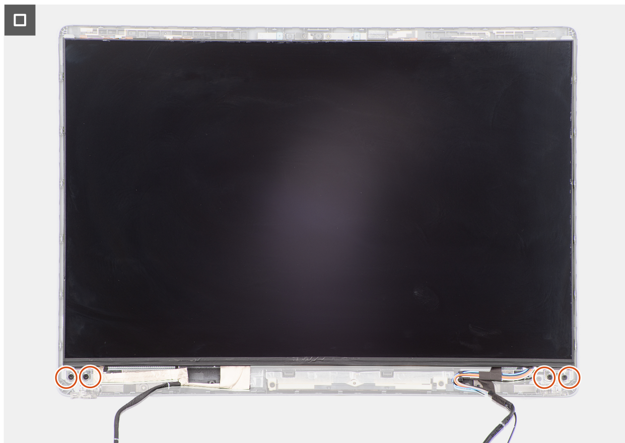
Figure 69. Installing the display panel
