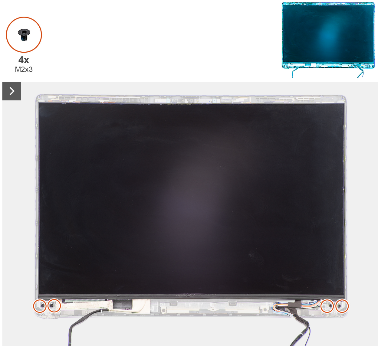
Figure 64. Removing the display panel
