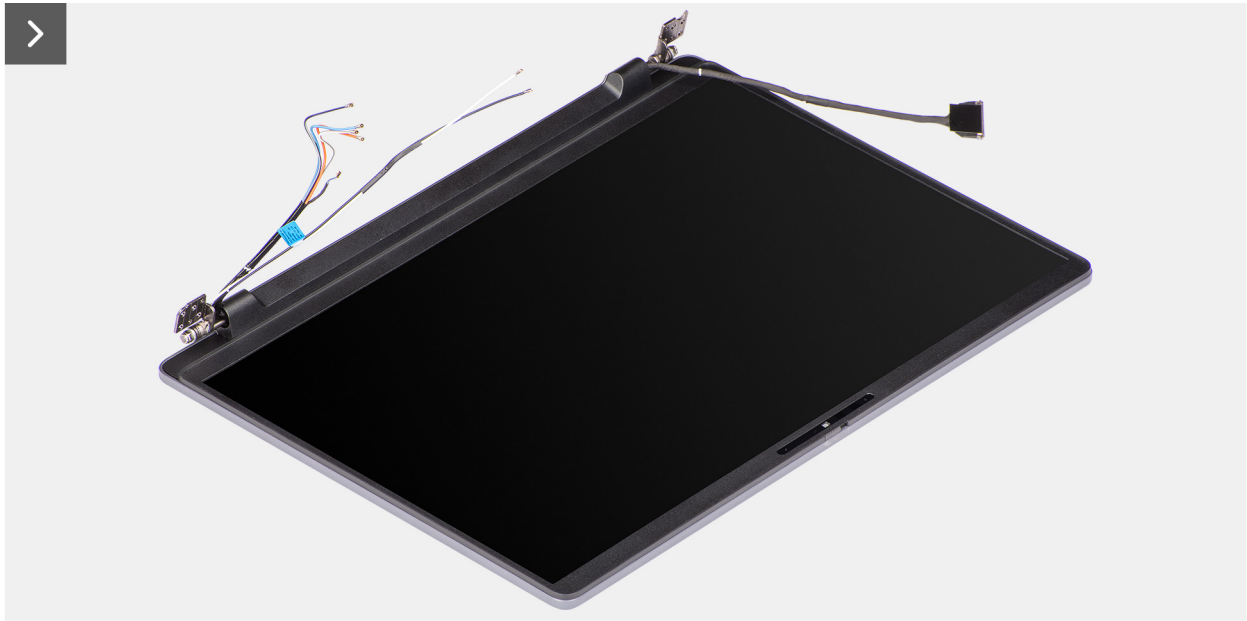
Figure 53. Installing the display assembly
