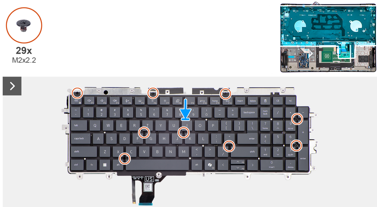
Figure 90. Installing the keyboard
