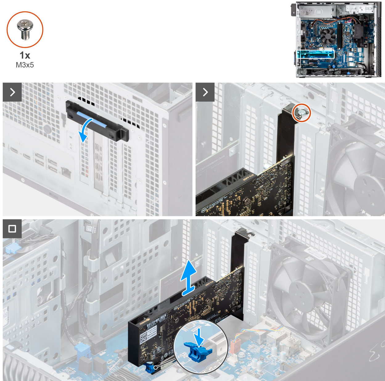
Figure 37. Removing the graphics card
