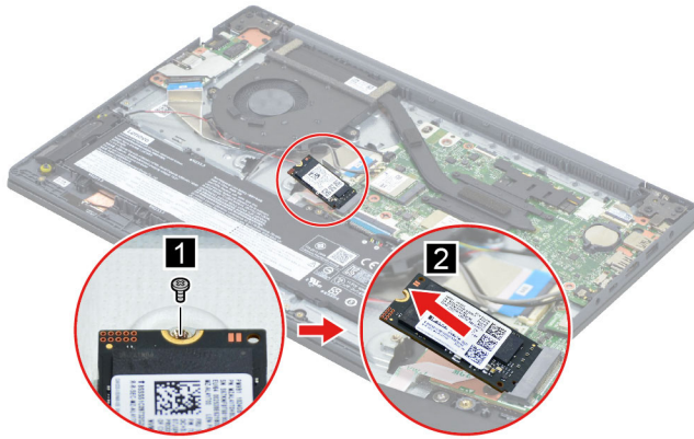
Figure 79. Remove one screw then remove the SSD by pulling it away from the slot
