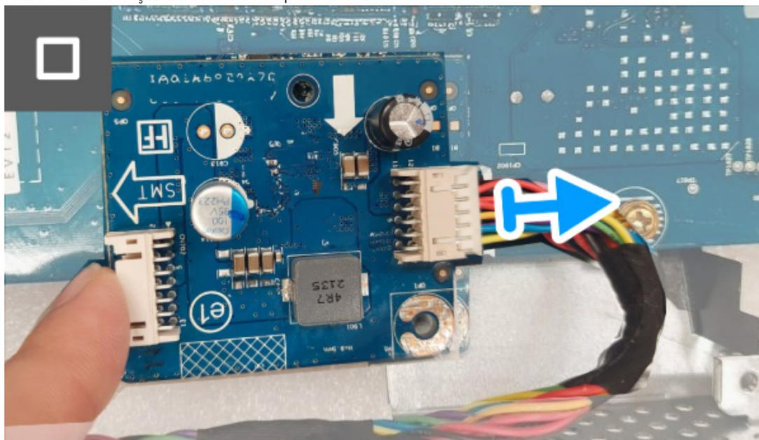
**Figura 25. Remover a placa DC-DC**
