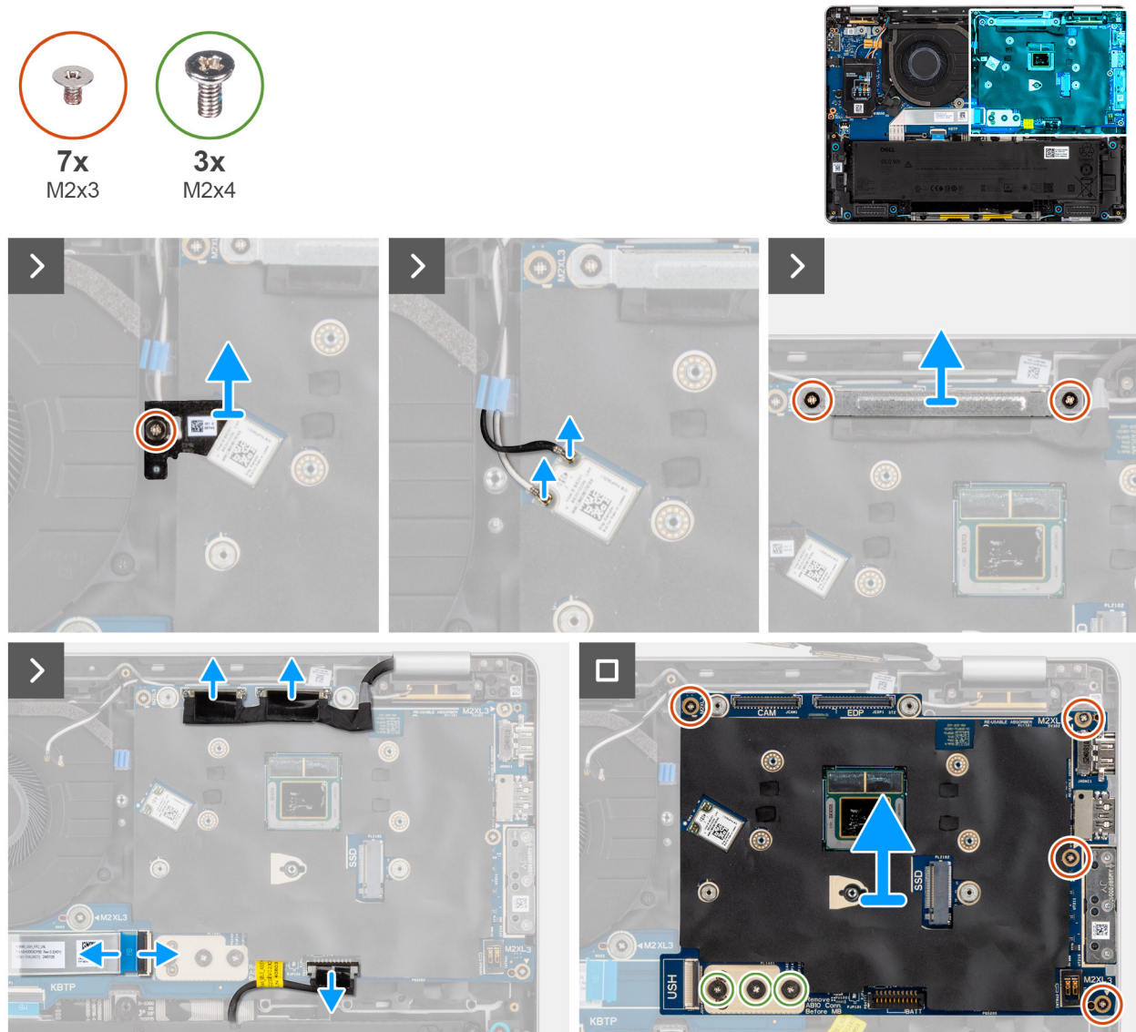
Figure 47. Removing the system board
