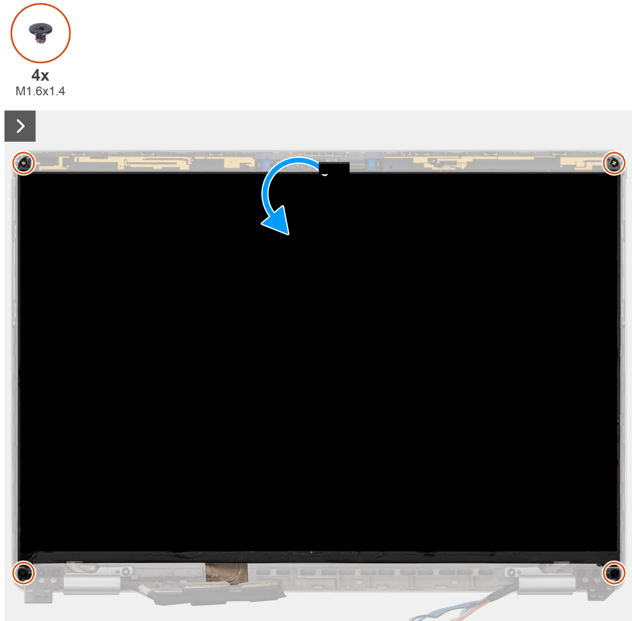
Figure 67. Removing the display panel
