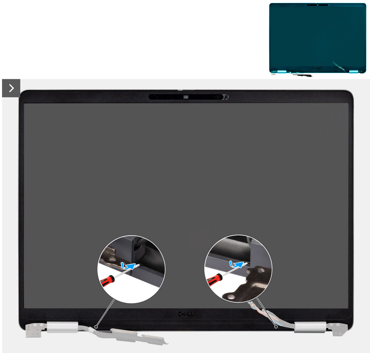
Figure 60. Removing the display bezel
