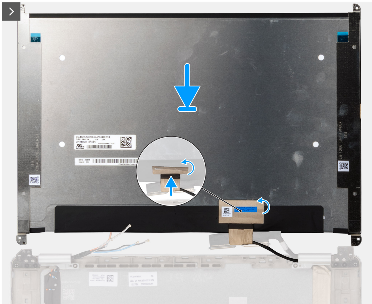
Figure 70. Installing the display panel
