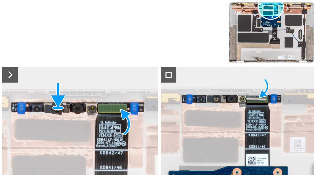
Figure 77. Installing the MIPI camera
