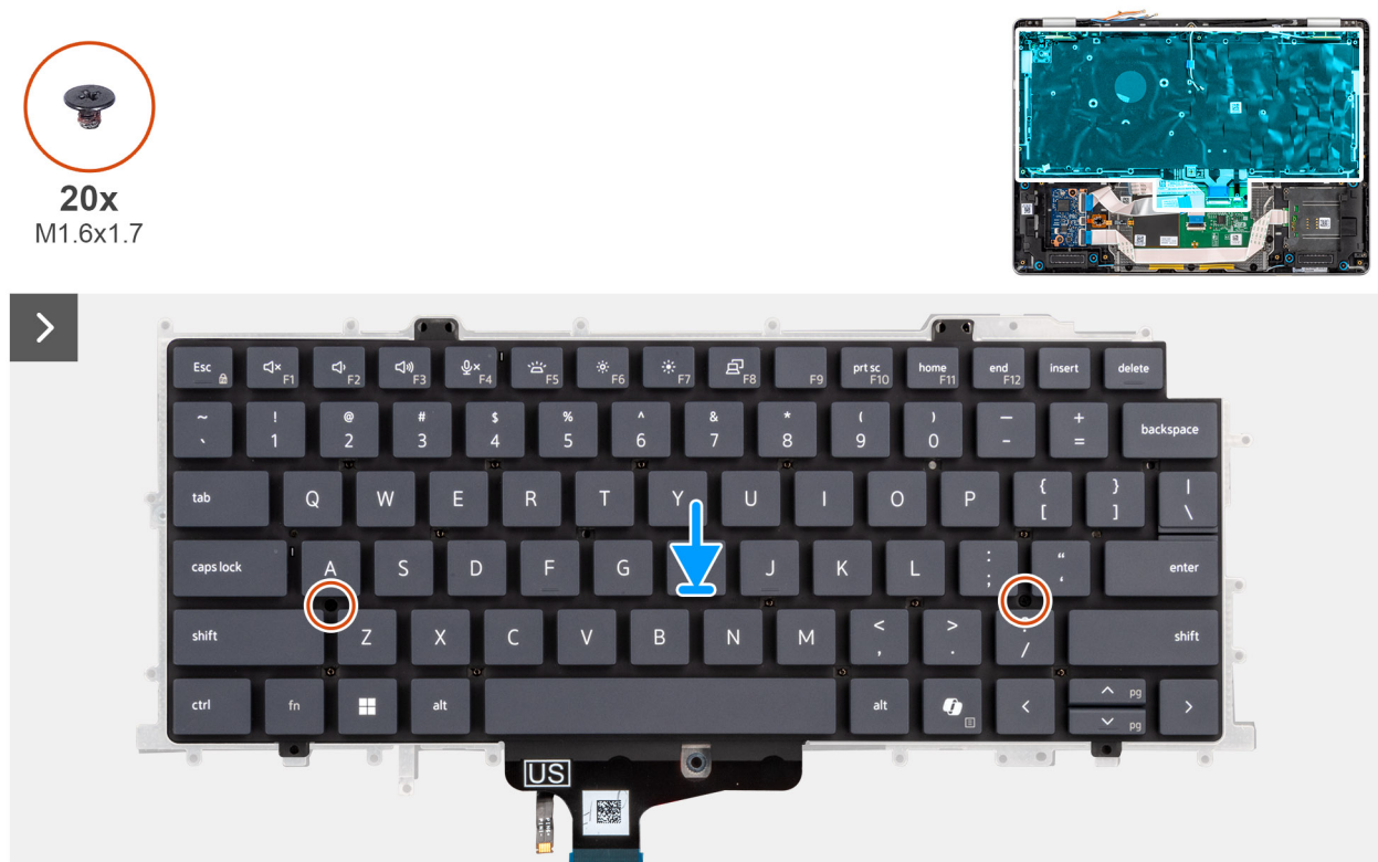
Figure 82. Installing the keyboard
