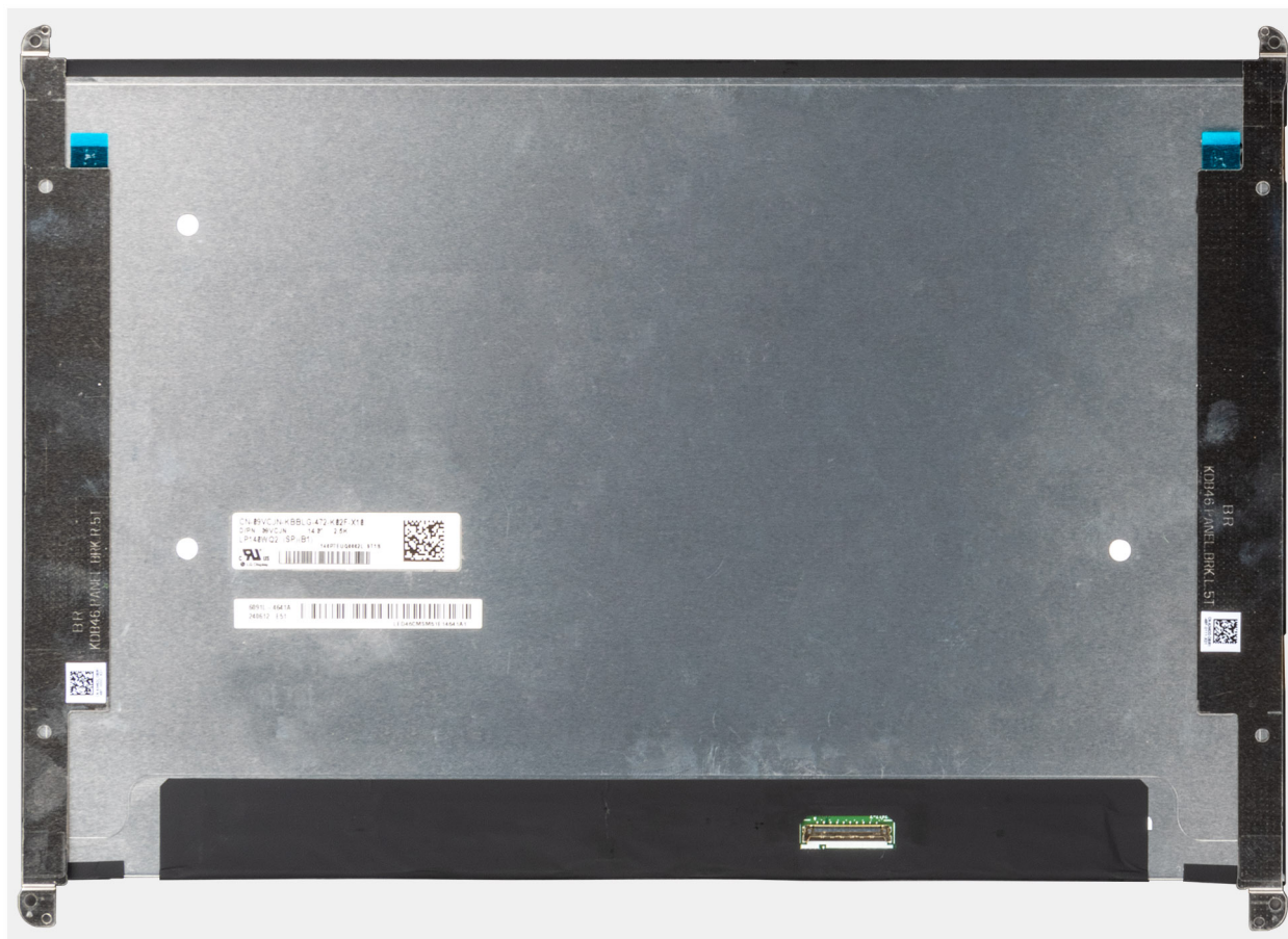
Figure 69. Display panel with brackets
