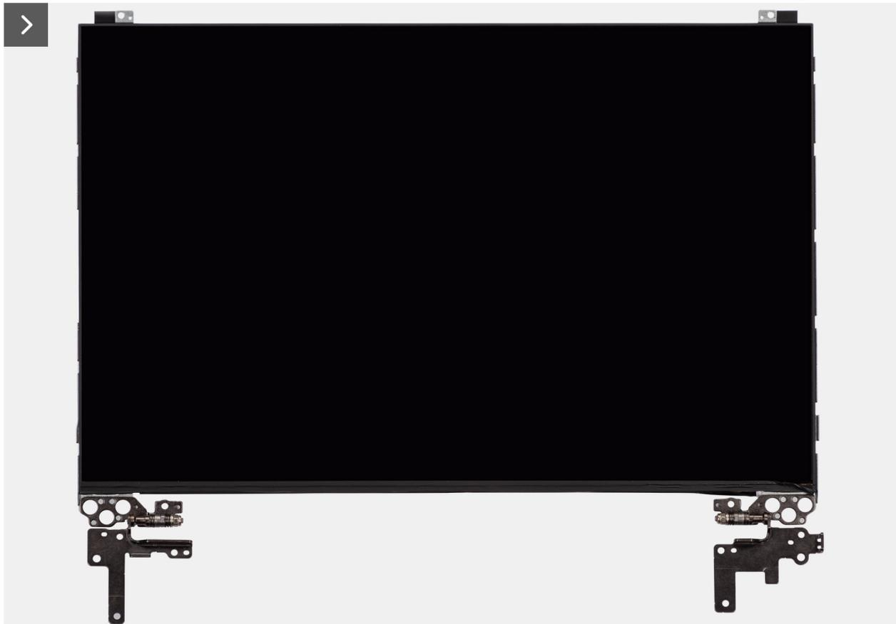
Figura88. Installing the display-panel assembly
