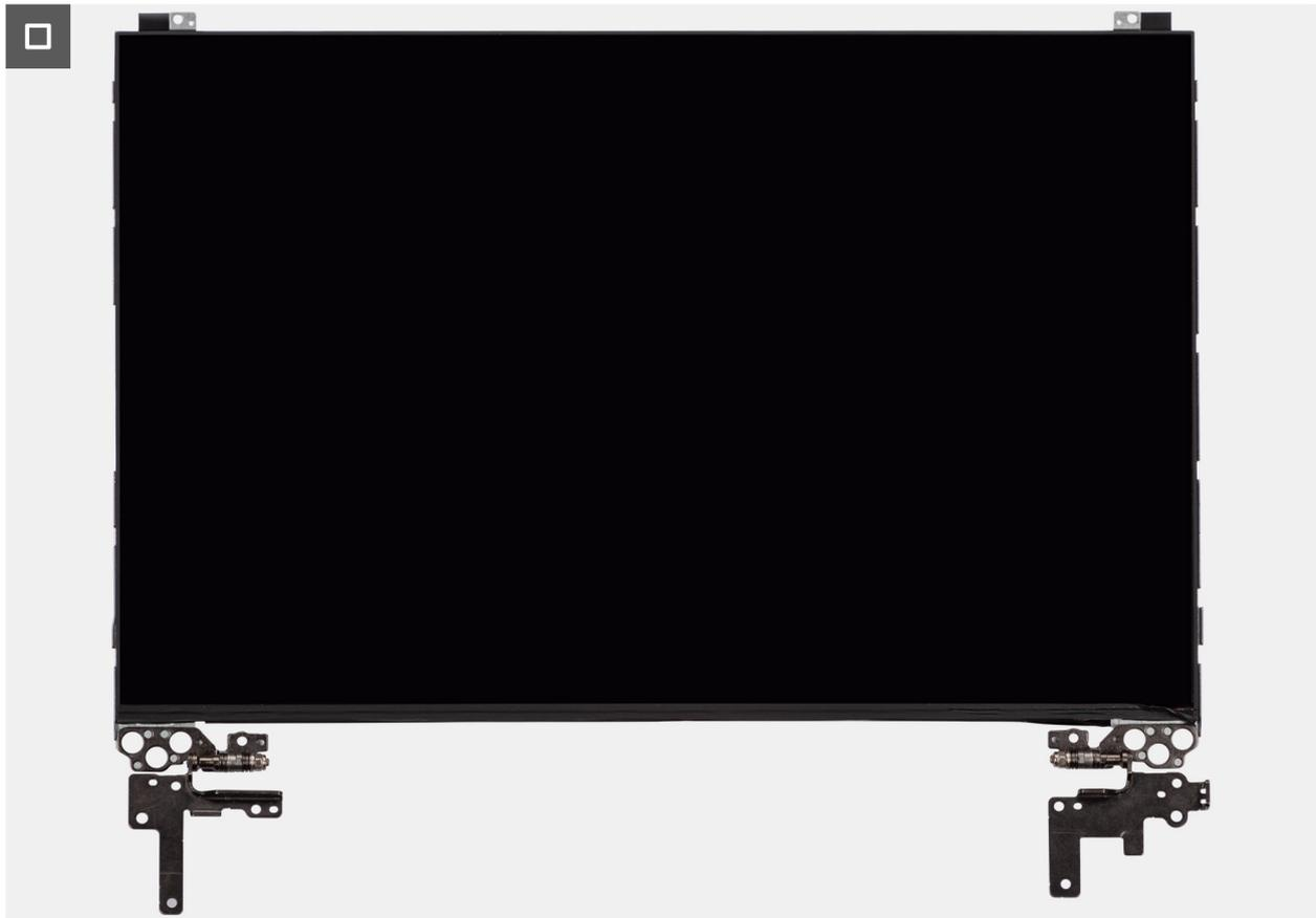
**Figura87. Removing the display-panel assembly**
