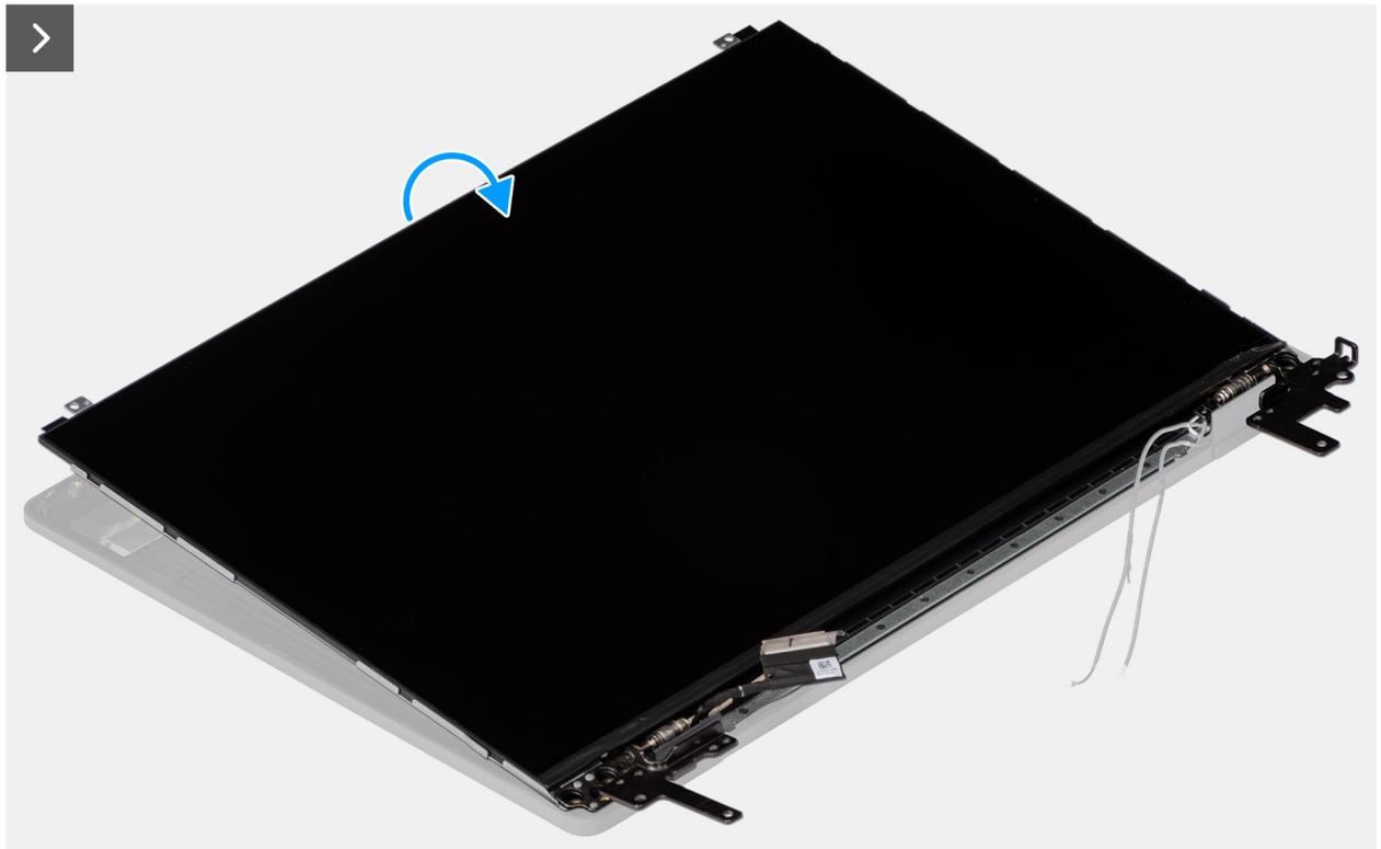
Figura85. Removing the display-panel assembly
