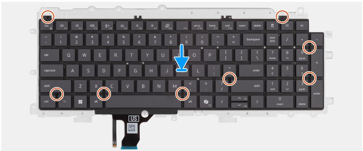
Figura69. Installing the keyboard support plate
