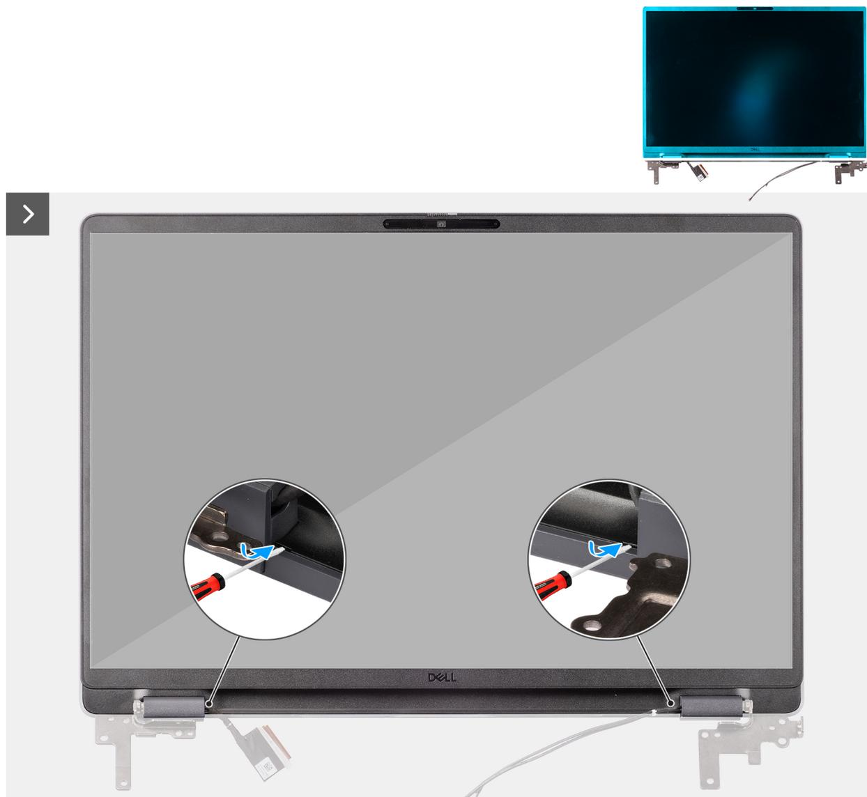
Figura77. Removing the display bezel
