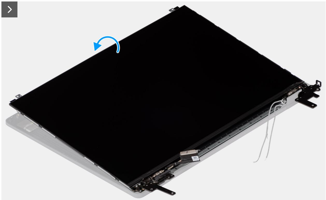
Figura90. Installing the display-panel assembly
