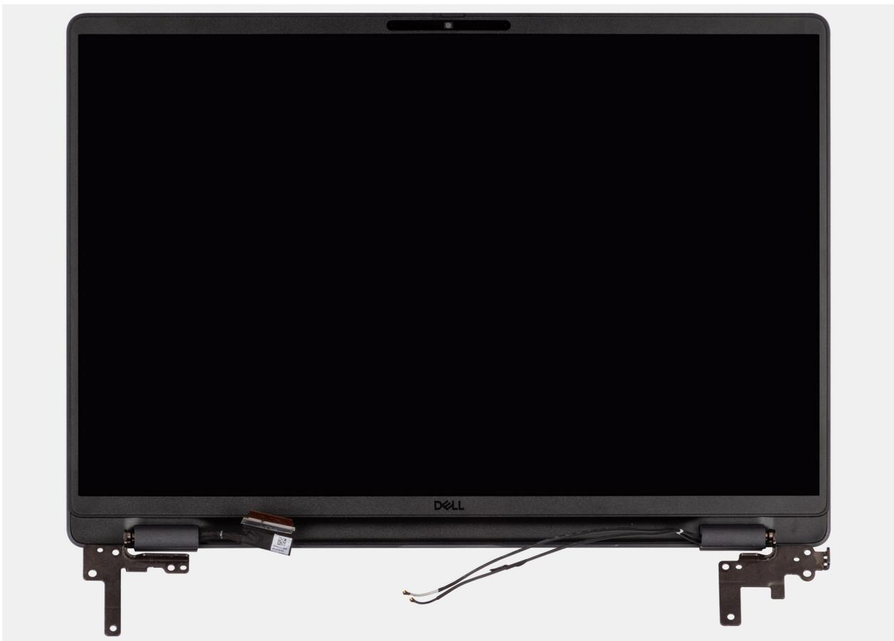
Figura74. Removing the display assembly
