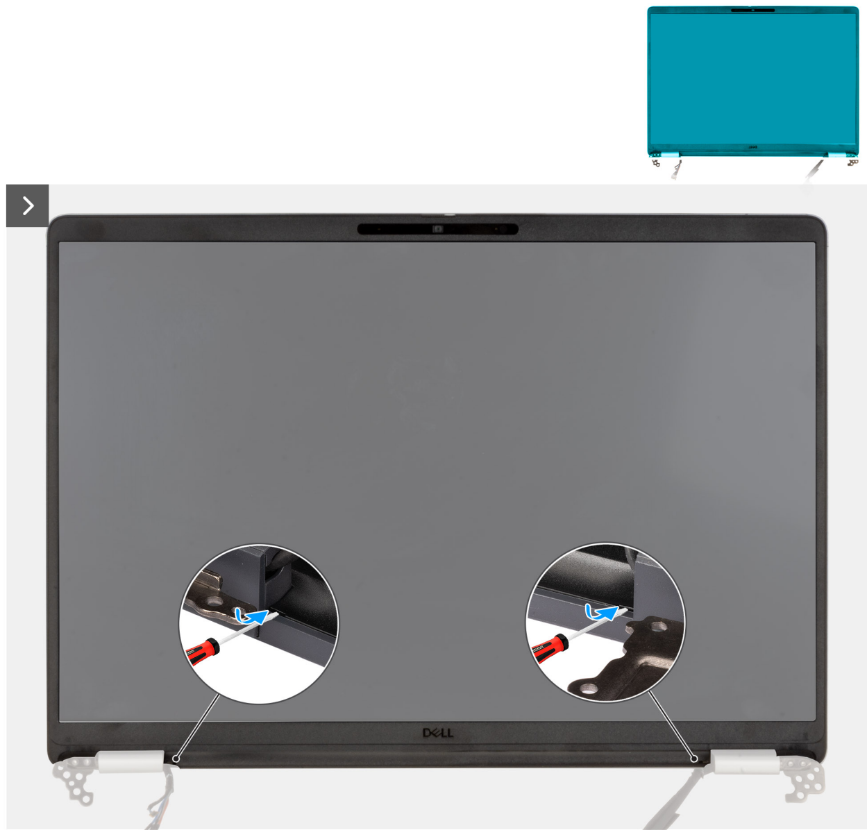
Figure 59. Prying the plastic bezel
